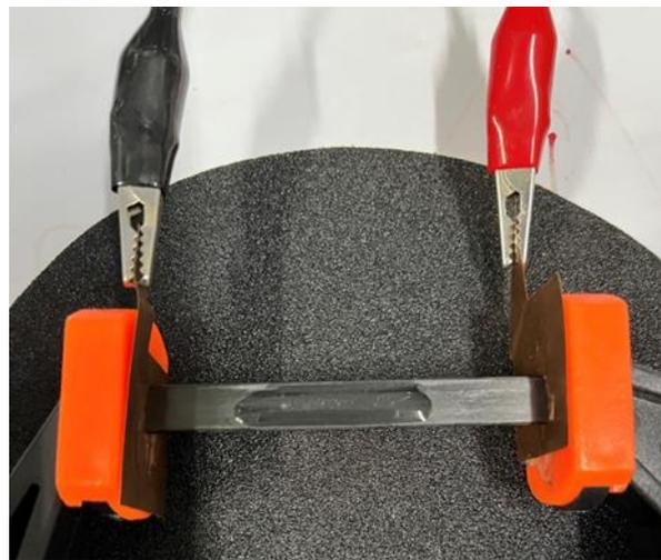
**Figure 8.** The experimental set-up for the deicing test of the CF/EP composite plate.
