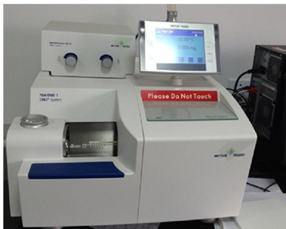
Figure 5. Thermogravimetric analyzer.
