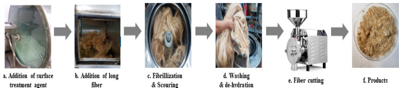
Figure 7. Process of surface treatment for natural fibers.
