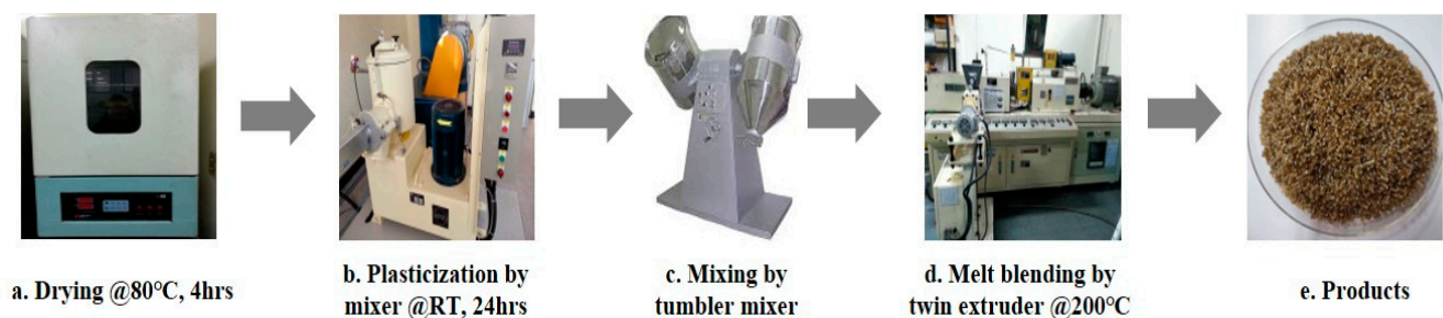
Figure 8. Process of preparing the cellulose acetate propionate–biofiller composite by melt blending.
