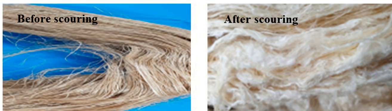
Figure 11. Before and after treatment of natural fiber.
