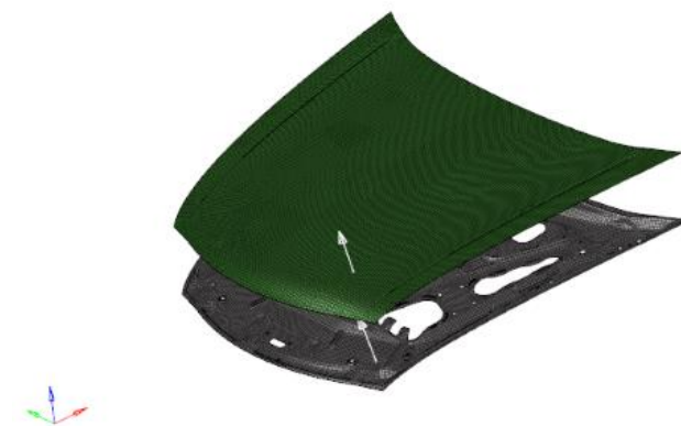
Figure 7. Model of CF/BF hybrid composites engine hood.
