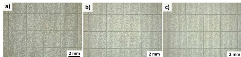
Figure 9. Microscopic images after the cross-cutting tests. PA12 coatings deposited by a constant energy density of 2.1 \text{ J/mm}^2 and different powder mass flows of (a) 0.2 \text{ g/min} , (b) 0.6 \text{ g/min} and (c) 1.4 \text{ g/min} .
