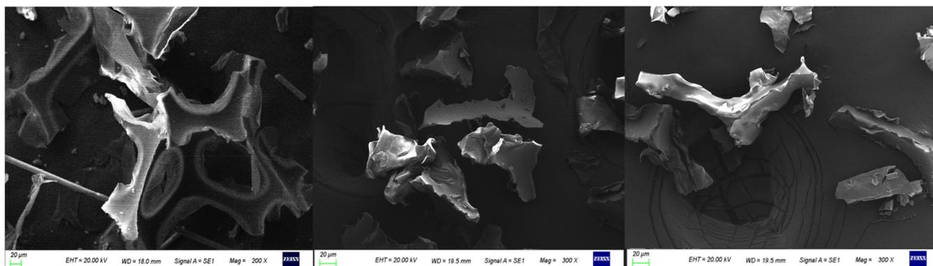
**Figure 8.** Microstructure of polyurethane powders with different mesh numbers: (a) 40 mesh, (b) 120 mesh, (c) 200 mesh.
