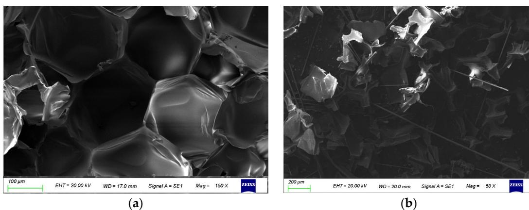
**Figure 7.** Microstructure of polyurethane before and after crushing, (a) before crushing, (b) after crushing.
