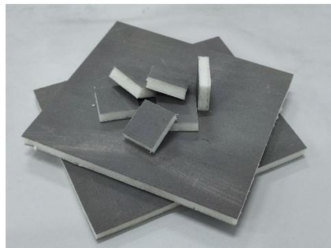
**Figure 1.** Waste rigid polyurethane insulation board.
