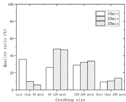
**Figure 4.** Particle size distribution for different times at 5000 r/min.
