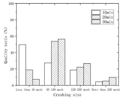
**Figure 2.** Particle size distribution for different times at 3000 r/min.
