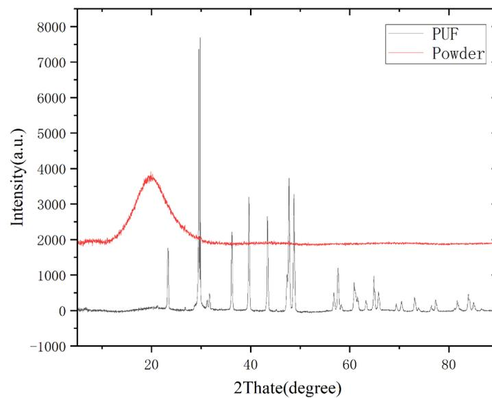
**Figure 6.** XRD curves before and after crushing.
