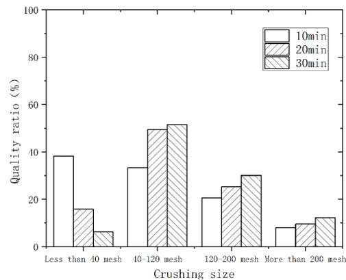
**Figure 3.** Particle size distribution for different times at 4000 r/min.
