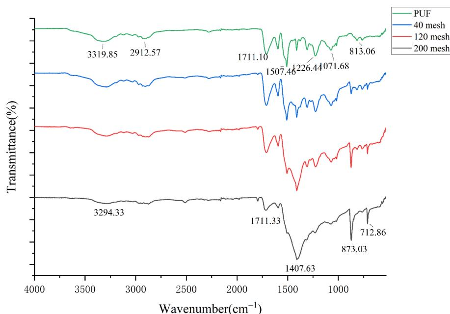
**Figure 5.** Fourier infrared spectra of polyurethane powders with different mesh numbers.
