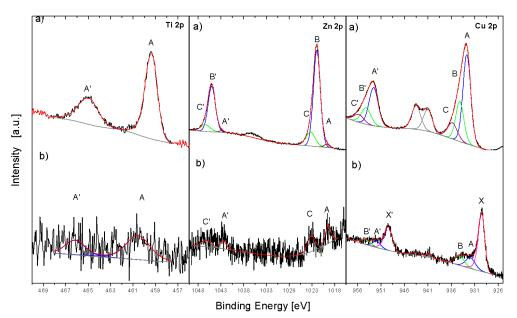
**Figure 3.** XPS analysis of the filler before (**a**) and after (**b**) interaction with PA12. The comparison of Cu 2p, Zn 2p and Ti 2p spectra.
