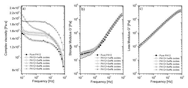
**Figure 5.** (a) Dynamic viscosity; (b) storage modulus G' and (c) loss modulus G'' as a function of frequency for pure PA12 and PA12 with the addition of 1–5 wt % metals oxides.
