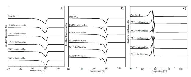
Figure 4. DSC curves for studied materials; (a) first heating; (b) second heating; (c) cooling.
