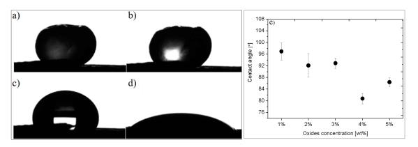
**Figure 2.** Images of the PA12 pellet melted at the filler surface: (**a**) original PA12 pellet; (**b**) first softening of the pellet at 150 °C; (**c**) completely melted PA12 at 180 °C; (**d**) wetting of the filler tablet by fully spread PA12 polymer at 224 °C; (**e**) dependence between contact angle of in PA12 composites and metal oxides concentration.
