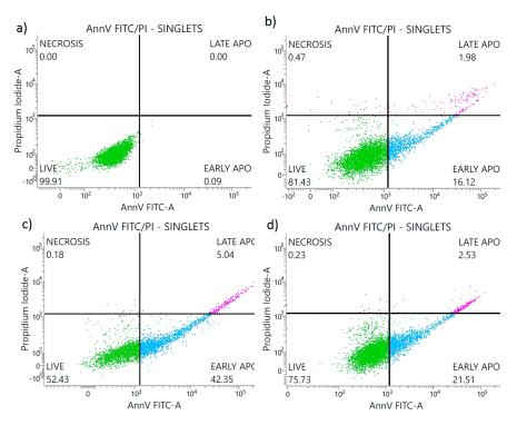
**Figure 7.** Percentage share of the L929 cells: alive, early apoptotic, late apoptotic and necrotic after 24 h treatment with: (a) DMEM—control group; (b) 4 h extract of pure PA12; (c) 4 h extract of PA12 with 3 wt % of metal oxides; (d) 4 h extract of PA12 with 4 wt % of metal oxides. The experiment was performed in triplicate.
