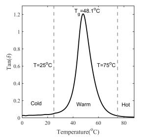
**Figure 7.** Tan  $\delta$  measured with DMA at a frequency of 1 Hz and a heating rate of 4 °C/min.
