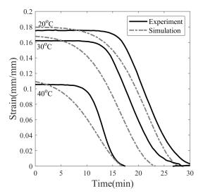
**Figure 14.** Shape recovery of SMP on heating at 4 °C/min after the isothermal recovery step at three different programming temperatures: 20, 30, and 40 °C.
