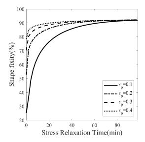
**Figure 19.** Effect of the stress relaxation time on the shape fixity of SMP at different programming strains ( $\epsilon_p$ ).
