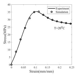
Figure 5. The stress–strain response of SMP deformed with a strain rate of 0.0013 s<sup>-1</sup> at T = 20 °C in the glassy state.
