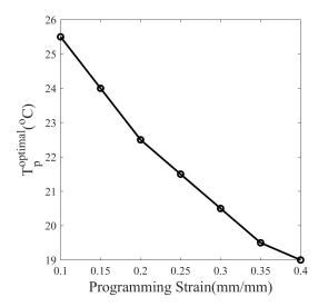
**Figure 18.** Dependence of optimum programming temperature  $(T_p^{optimal})$  on programming strain of the SMP.
