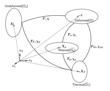
Figure 1. An analogous decomposition scheme for the deformation gradient.
