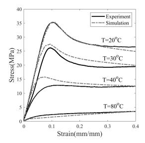
**Figure 8.** Stress response of uniaxial tension at a strain rate of  $0.0013 \text{ s}^{-1}$  of SMP at different temperatures.
