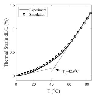
**Figure 3.** Evolution of thermal strain measured by DMA of SMP subjected to stress-free cooling at 4 °C/min.
