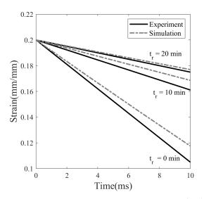
**Figure 16.** Instantaneous strain recovery on unloading for three different cases of stress relaxation times: 0, 10, and 20 min.
