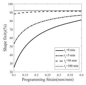
**Figure 20.** Effect of the programming strain on the shape fixation of SMP at different stress relaxation times  $(t_r)$ .
