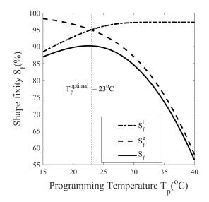
**Figure 17.** Variation of instantaneous, gradual, and overall shape fixity measured after the isothermal recovery step of thermomechanical cycles performed at programming temperatures ranging from 15 to 40 °C.
