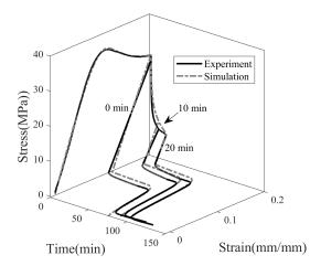
**Figure 15.** Thermomechanical behaviour of SMP at three different stress relaxation times: 0, 10, and 20 min (with  $\epsilon_p = 0.2$ ,  $T_p = 20$  °C).
