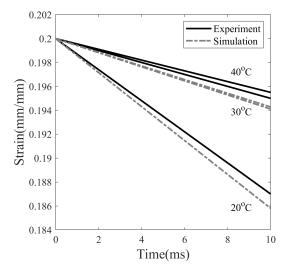
**Figure 12.** Instantaneous strain recovery of SMP at three different programming temperatures: 20, 30, and 40 °C due to unloading.
