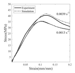
**Figure 6.** The stress–strain response of deformed SMP at strain rates of 0.0013 and 0.0039  $s^{-1}$ .
