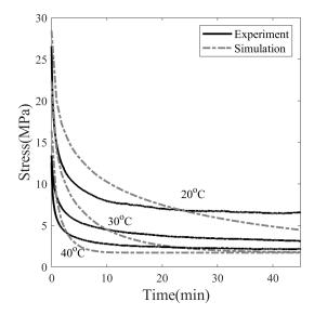
Figure 11. Effect of programming temperature on stress relaxation of SMP at 20% pre-strain.
