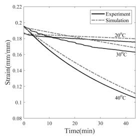
**Figure 13.** Stress-free isothermal recovery of SMP at temperatures 20, 30, and 40 °C after fixation of the temporary shape.
