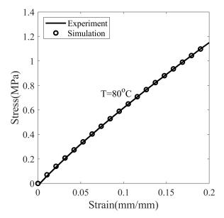
**Figure 4.** The stress–strain response of SMP deformed with a strain rate of 0.0013 s<sup>-1</sup> at T = 80 °C in the rubbery state.
