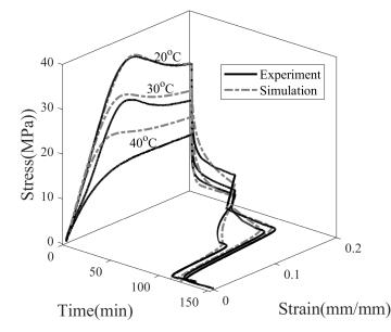
**Figure 10.** Thermomechanical behavior of SMP at programming temperatures, 20, 30, and 40 °C (with  $\epsilon_p = 0.2$ ,  $t_r = 45$  min).
