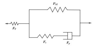
Figure 2. A linear thermoviscoelastic rheological model.
