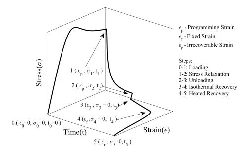
**Figure 9.** Representation of steps involved in the thermomechanical cycle in cold programming of SMP.
