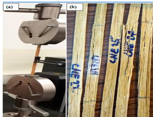
**Figure 4.** (a) Set-up of the tensile test machine; (b) mode of failure.
