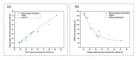
**Figure 3.** (a) Correlation between steady-state and TPS thermal conductivity experimental values; (b) difference percentage between TPS and steady-state methods as a function of the thermal conductivity.
