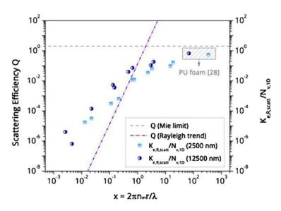
**Figure 6.** Right axis: Scattering efficiency *Q* for a Rayleigh-like behaviour and Mie limit as a function of the size parameter *x*. Left axis: Scattering extinction coefficient normalized by the 1D cell density as a function of the size parameter *x*. (Reprinted with permission from Ref. [101], Copyright © 2020, Elsevier).
