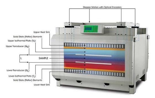
Figure 2. Heat flow meter measurement scheme [26].
