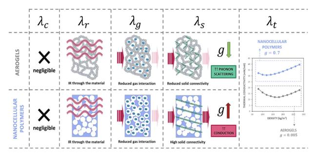
**Figure 8.** Heat transfer mechanisms in aerogels and nanocellular polymers. While both systems behave similarly in terms of radiation and conduction through the gas phase, there is a huge difference in the conduction through the solid material due to the intrinsic configuration of the solid phase. Nanocellular polymers show a connected solid phase, and as a result, higher conductivity.
