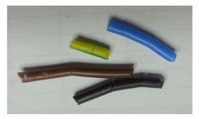
Figure 5. Appearance of cracks in XLPE insulations (IC1 cable) after three years of irradiation in SPS.
