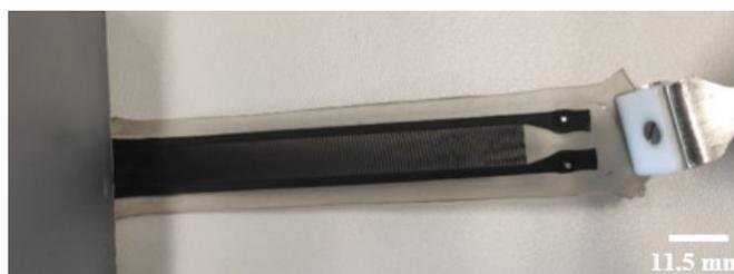
**Figure 17.** Sensor patch developed with batch manufacturing process II after 1000 motion cycles.
