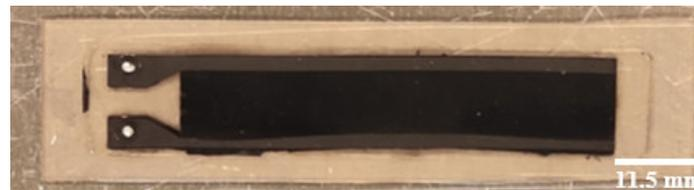
**Figure 9.** Flexible capacitive strain Gauge sensor produced with batch manufacturing process II.
