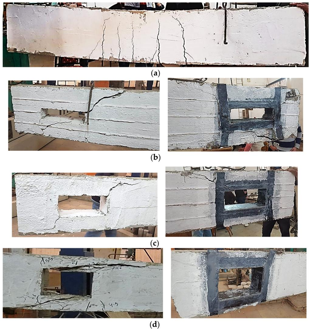
Figure 8. Failure Model of Samples with Shear-Zone Openings. (a) control beam; (b) opening  $90 \times 360 \text{ mm}^2$ ; (c) opening  $150 \times 360 \text{ mm}^2$ ; (d) opening  $210 \times 360 \text{ mm}^2$ .
