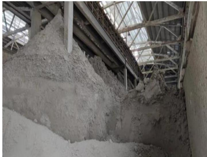
**Figure 1.** Iron-ore tailings for test.
