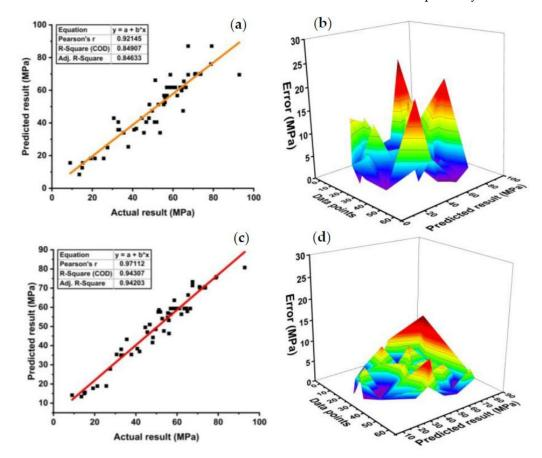
**Figure 7.** DT model results for compressive strength; (**a**) individual regression model, (**b**) error distribution between actual and target values of individual model, (**c**) ensemble regression model, (**d**) and error distribution between actual and target values of an ensemble model.
