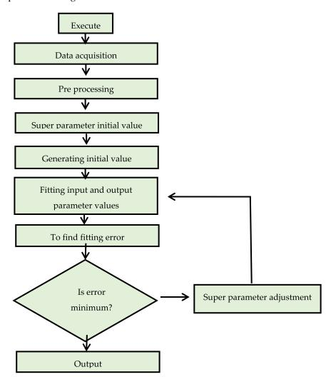
Figure 4. Flow chart of Support Vector Machine.
