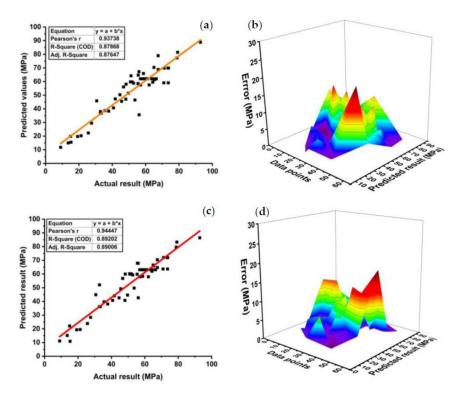
**Figure 8.** SVM model results for compressive strength; (**a**) individual regression model, (**b**) error distribution between actual and target values of individual model, (**c**) ensemble regression model, and (**d**) error distribution between actual and target values of an ensemble model.
