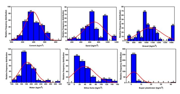
**Figure 5.** Relative frequency distribution of parameters to compressive strength; cement, sand, gravel, water, silica fume, and super plasticizer.
