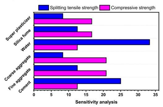
Figure 10. Contribution of input parameters to compressive and splitting tensile strength.
