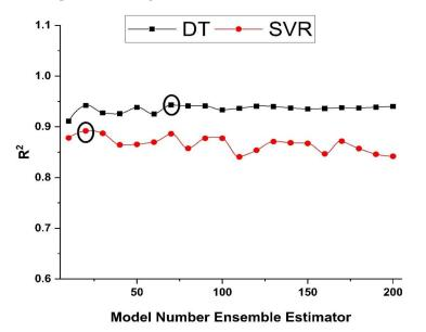
**Figure 6.** Coefficient of determination for ensemble models with the various number of component sub-models for compressive strength.
