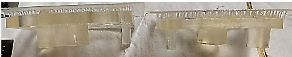
**Figure 5.** The clear parts printed with 10 s for heavy structure in the left position and 8 s for medium structure in the right position.
