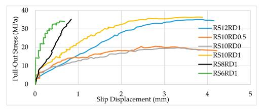
**Figure 4.** Pull-out stress showing stress versus slip for 10 mm diameter BFRP bars, with l = 10D and various rib spacings (RS) and rib depths (RD).
