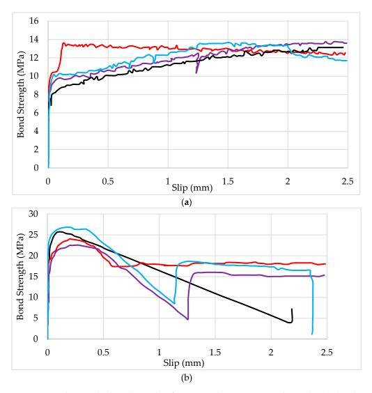
**Figure 5.** Bond strength–slip relationship for 10-mm diameter wrapped samples (each color is different sample) BFRP bars with (a) primary sand coating, (b) secondary sand coating. Reprinted with permission from ref. [27]. Copyright 2021 Elsevier Science & Technology Journals.
