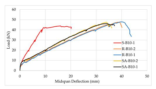
Figure 7. Steel-reinforced beam (S-B10-1) is much stiffer than similar BFRP-reinforced beams.
