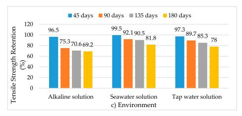
**Figure 9.** Tensile strength retention in 8 mm diameter FRP bars made of vinyl ester matrix subjected to three environments with bars made of (a) BFRP fibers, (b) CFRP fibers, (c) GFRP fibers. Reprinted with permission from ref. [48]. Copyright 2021 American Society of Civil Engineers
