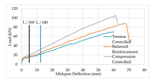
**Figure 6.** Load–deflection relationship for beams reinforced with BFRP bars and BFRP stirrups Reprinted with permission from ref. [16]. Copyright 2021 American Society of Civil Engineers.
