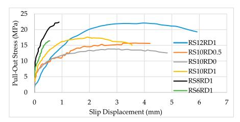
**Figure 3.** Pull-out test result showing stress versus slip for 10 mm diameter BFRP bars with bond length l = 5D with various rib spacings and rib depths. RS12RD1 = Rib spacing of 12 mm and rib depth of 1 mm. Reprinted with permission from ref. [21]. Copyright 2021 ASTM International.
