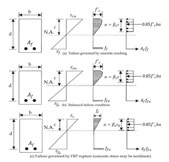
Figure 8. Strain and stress distribution at ultimate conditions [2].
