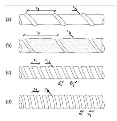
**Figure 2.** Fiber-reinforced polymers (FRP) bar surface configurations: (a) Ribbed and helically wrapped, (b) ribbed, helically wrapped, and sand coated, (c) indented, (d) ribbed.
