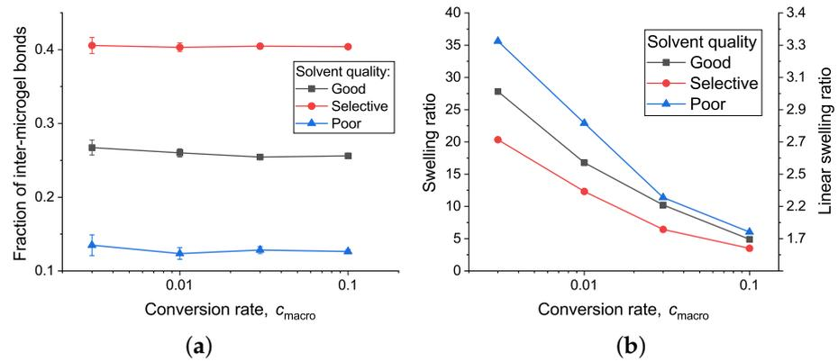
**Figure 5.** Dependence of fraction of bonds between neighbor microgels  $\varphi$  (a) and swelling or linear swelling ratio (b) on conversion rate for systems crosslinked in various types of solvent. Statistical errors that exceed points size are shown in bars.
