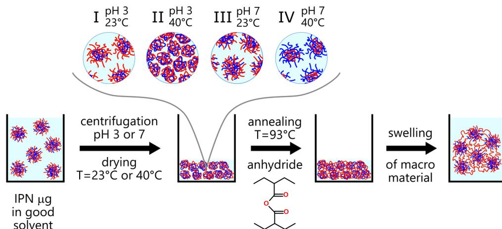
**Figure 1.** Scheme of the formation of material from microgels. IPN particles consist of two independent but topologically entangled networks: PNIPAM (red) and PAA (blue).
