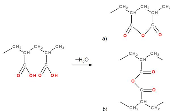
**Figure 2.** The reaction of the formation of polyacrylic acid anhydride with the formation of (a) intramolecular and (b) intermolecular structures.
