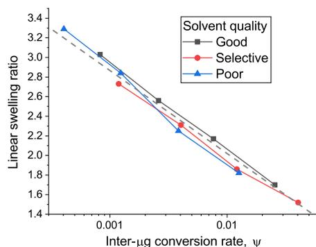
**Figure 7.** Linear swelling ratio for systems crosslinked in various types of solvent as a function of inter-microgel conversion rate. Statistical errors do not exceed the size of the points.
