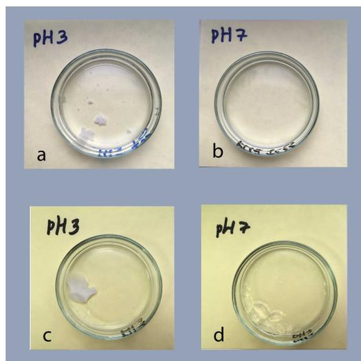
**Figure 3.** Photographs of macromaterials based on IPN microgels obtained by annealing from concentrated dispersions dried at 23 °C (a,b) and at 40 °C (c,d), and at pH 3 (a,c) and 7 (b,d).
