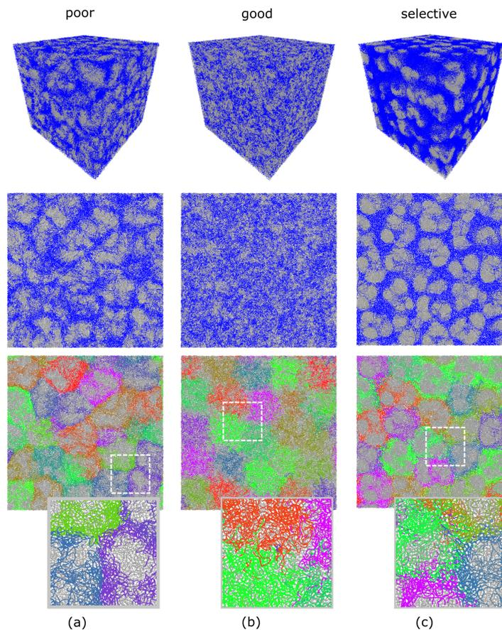
**Figure 6.** Snapshots of the simulated systems at concentration  $c = 0.9$  before crosslinking: in poor solvent (a), in good solvent (b), and in selective solvent (c). First and second rows are colored by non-crosslinking (gray) and crosslinking (blue) networks. In third row, non-crosslinking networks are drawn in grey, and crosslinking networks of individual microgel particles are shown in different colors.
