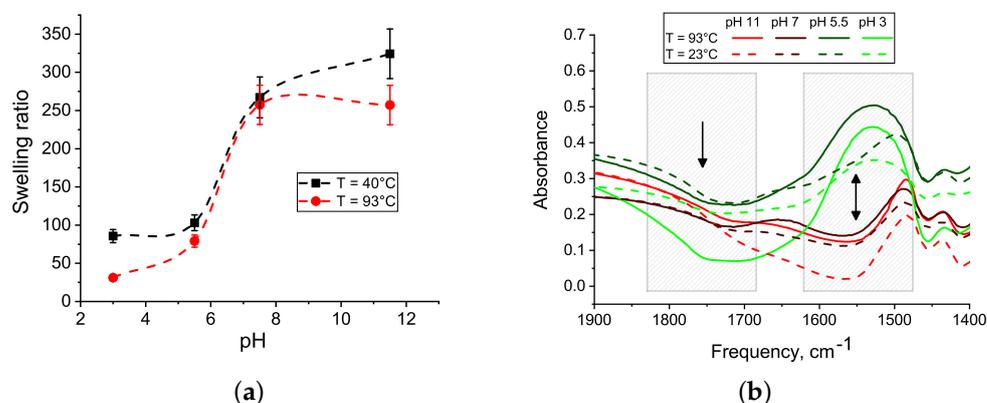
**Figure 4.** (a) Dependence of the equilibrium degree of swelling of PAA films on pH and annealing temperature, the lines are drawn to guide the eye. (b) IR spectra of linear PAA dried under different conditions.
