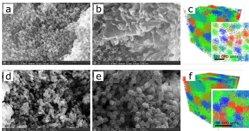
**Figure 8.** SEM microphotographs of microgel macromaterial cross-sections; (a, b) obtained at pH 7, (d, e) obtained at pH 3. Snapshots of the simulated systems with  $c_{\text{macro}} = 0.003$  (c) and  $c_{\text{macro}} = 0.1$  (f) after swelling, colored by individual microparticles.
