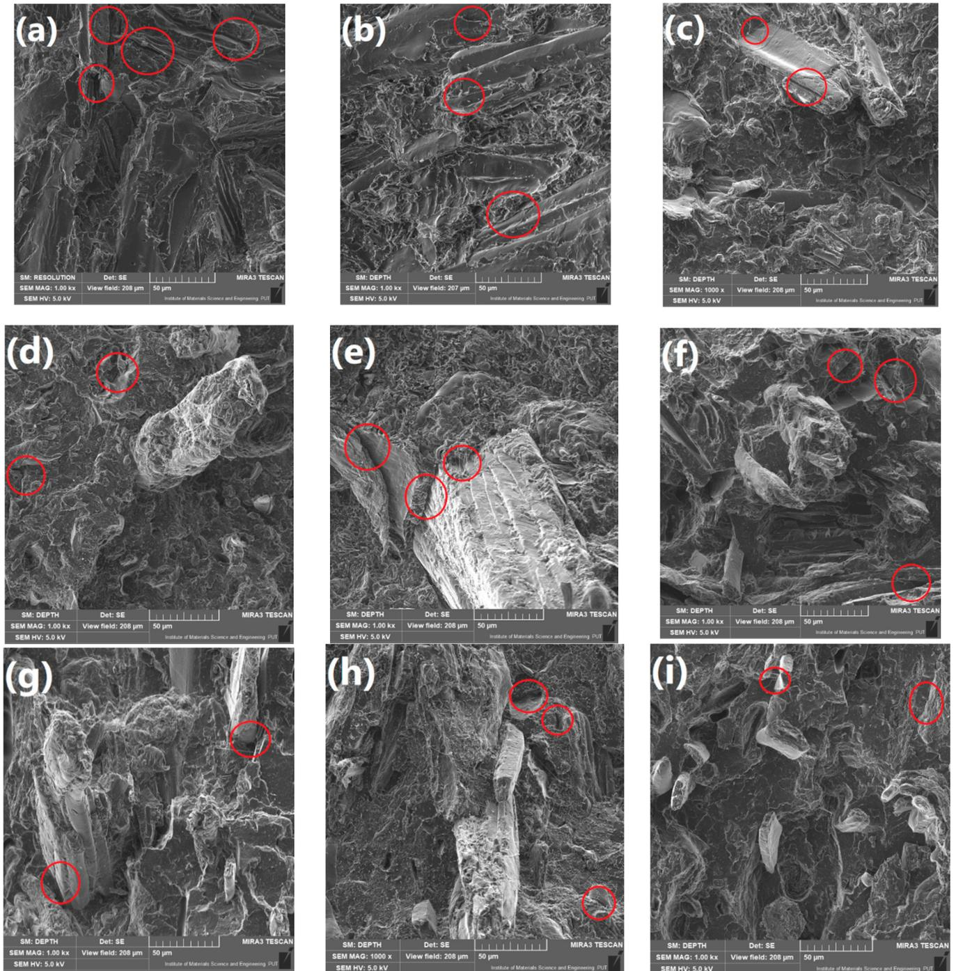
**Figure 4.** SEM images of brittle fracture areas of samples (a) WF<sub>100</sub>, (b) WF<sub>75</sub>BSG<sub>25</sub>, (c) WF<sub>50</sub>BSG<sub>50</sub>, (d) WF<sub>25</sub>BSG<sub>75</sub>, (e) WF<sub>0</sub>BSG<sub>100</sub>, (f) WF<sub>75</sub>LK<sub>25</sub>, (g) WF<sub>50</sub>LK<sub>50</sub>, (h) WF<sub>25</sub>LK<sub>25</sub>, and (i) WF<sub>0</sub>LK<sub>100</sub> under magnification of  $\times 1000$ .
