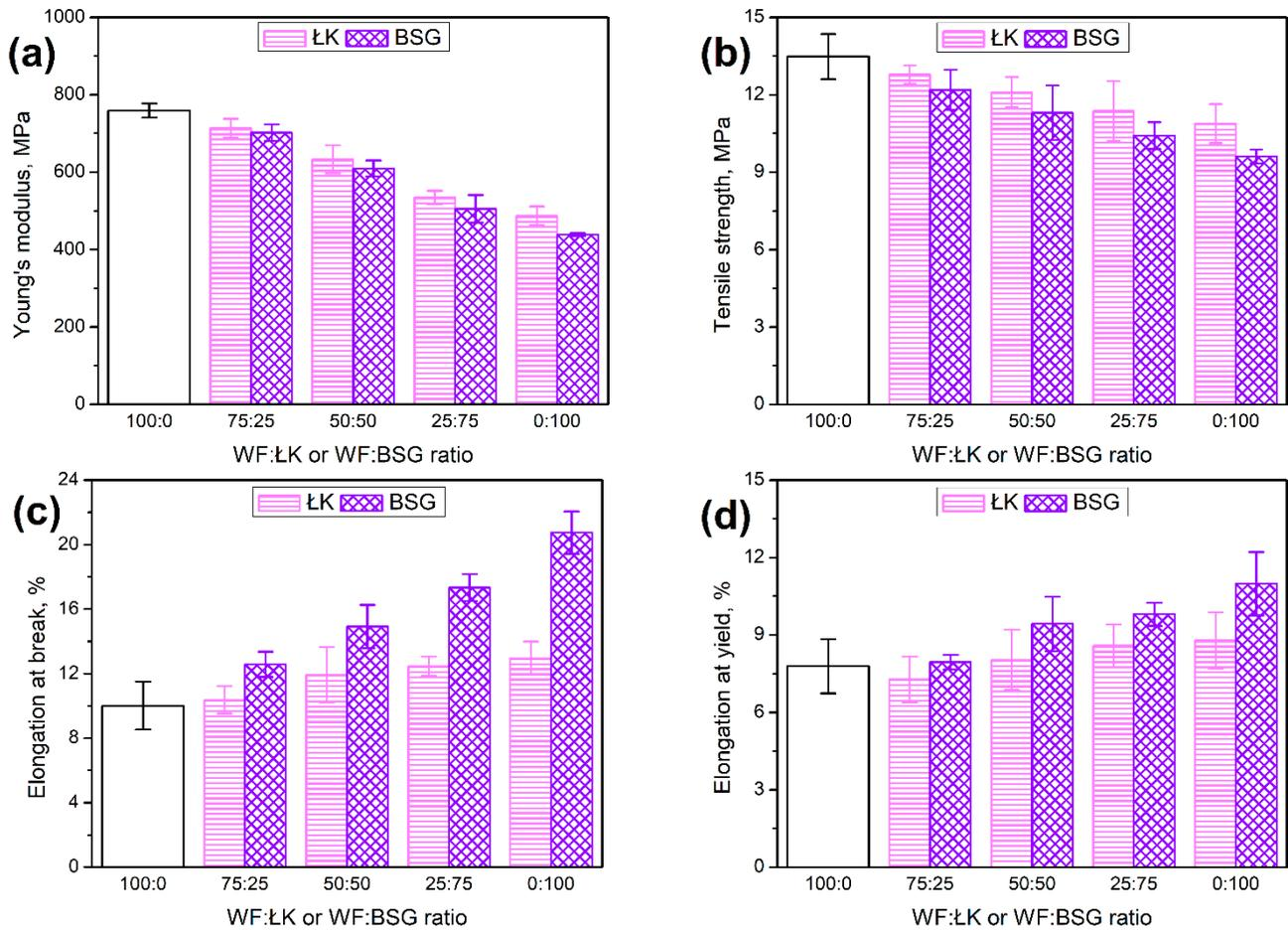
**Figure 7.** The effect of WF substitution with LK and BSG on the (a) Young's modulus, (b) tensile strength, (c) elongation at break, and (d) elongation at yield of prepared composites.
