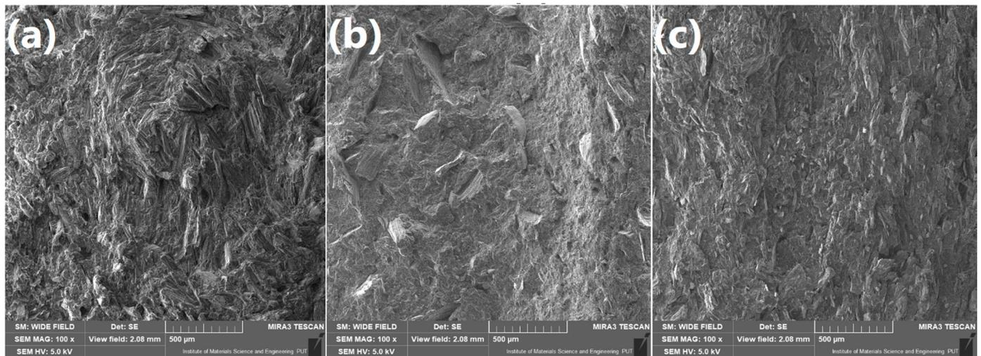
Figure 6. SEM images of brittle fracture areas of samples (a) WF<sub>100</sub>, (b) WF<sub>0</sub>BSG<sub>100</sub>, and (c) WF<sub>0</sub>LK<sub>100</sub> under magnification of  $\times 100$ .
