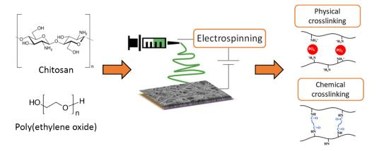
Figure 2. Schematic of the fabrication procedure of chitosan-based membranes.
