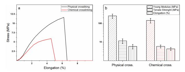
**Figure 4.** (a) Stress-deformation curves obtained from uniaxial tensile test for physically (black squares) and chemically crosslinked (red circles) electrospun mats. (b) Summary of the calculated mechanical properties (i.e., Young modulus E, elongation at break  $\varepsilon_{b}$ , and tensile strength  $\sigma_{b}$ ).
