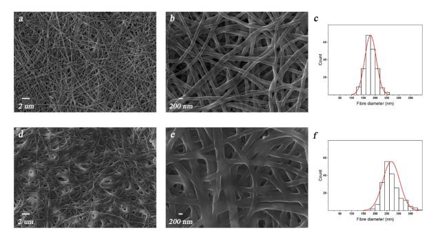
**Figure 3.** FESEM micrographs for chitosan membranes after (**a**,**b**) a physical or (**d**,**e**) a chemical crosslinking treatment and (**c**,**f**) their related size histograms.
