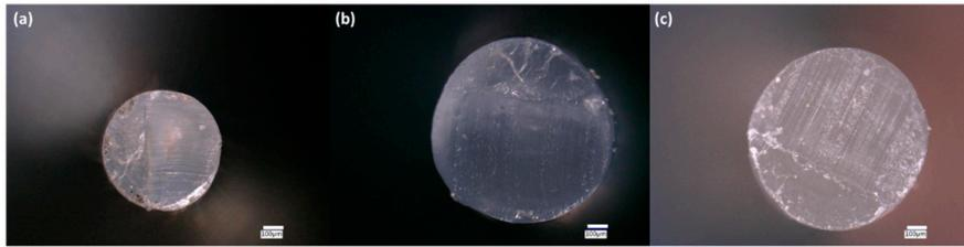
**Figure 2.** Digital microscopy cross-section images of: (a) PLA/PEG1k 90/10; (b) PLA/PEG2k 90/10; and (c) PLA/PEG10k 90/10.
