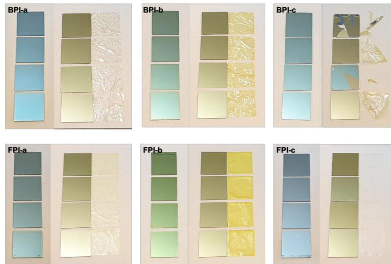
**Figure 1.** Ablation behavior of the prepared PI films before and after the XF-LO process. (The exposed XFL fluence, from top to bottom, were 0.85, 2.6, 4.2 and 5.8. J/cm<sup>2</sup>, respectively.).
