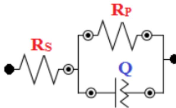
**Figure 7.** Equivalent circuit used for Nyquist plot analysis.
