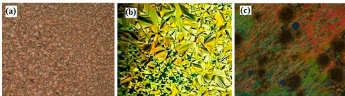
**Figure 5.** Textures under POM of the polymorphic phases for **A6/B10** SMHBC; (a) SmC phase at 110.0 °C; (b) SmA phase at 149.0 °C; (c) N phase at 180.0 °C.
