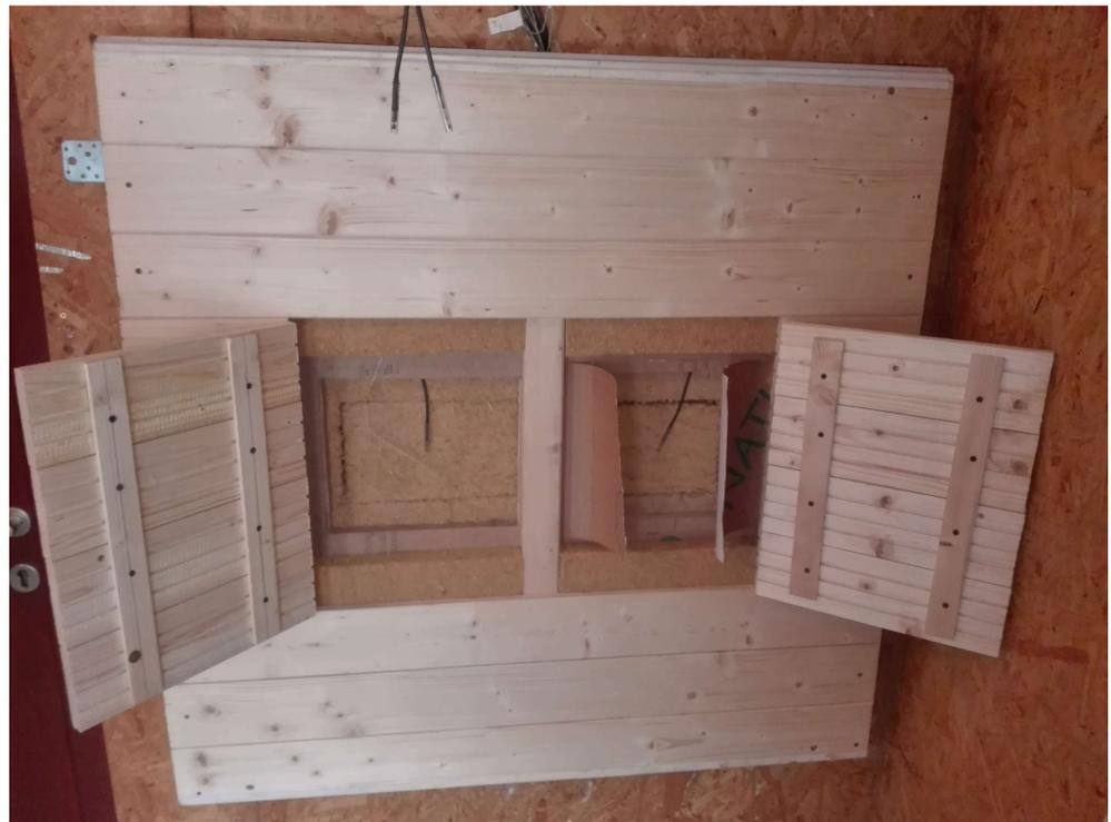
Figure 4. Log Wall LW1 and LW2 Installed in the Research Timber Structure, Interior.
