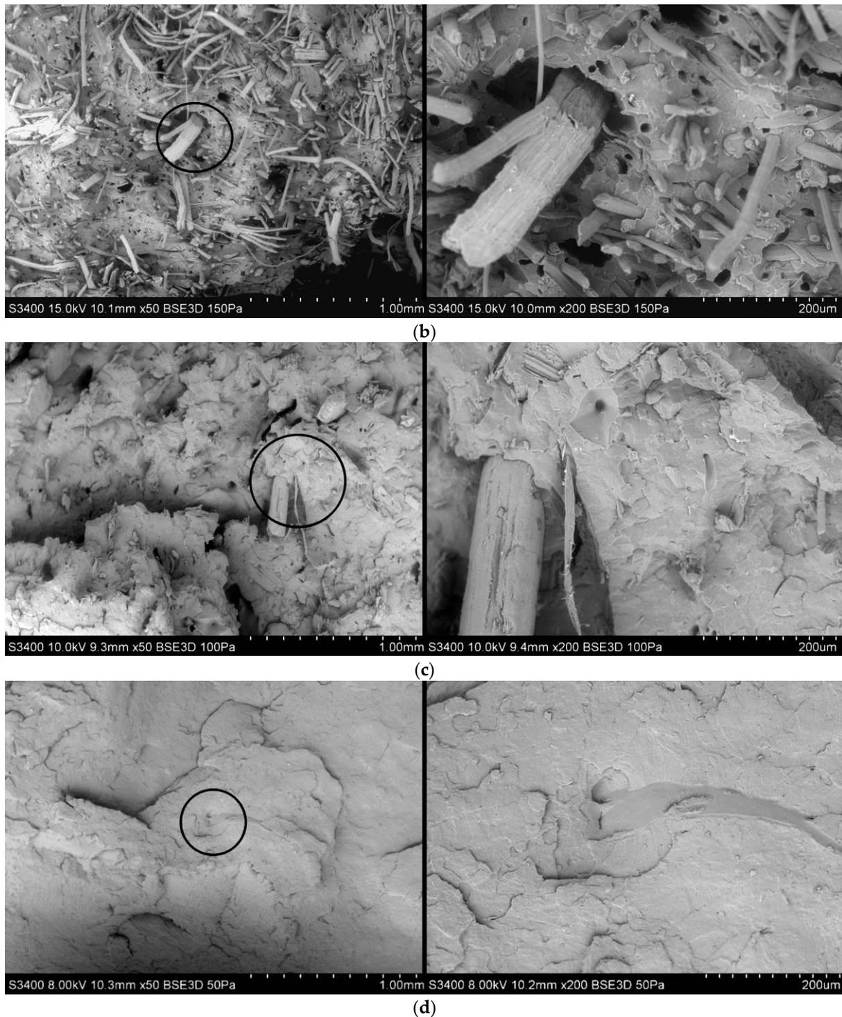
**Figure 10.** SEM photographs of fractures for biocomposites samples filled with fibers of (a) hemp, (b) flax and (c) wood; (d) SEM photograph for pure PHBV.
