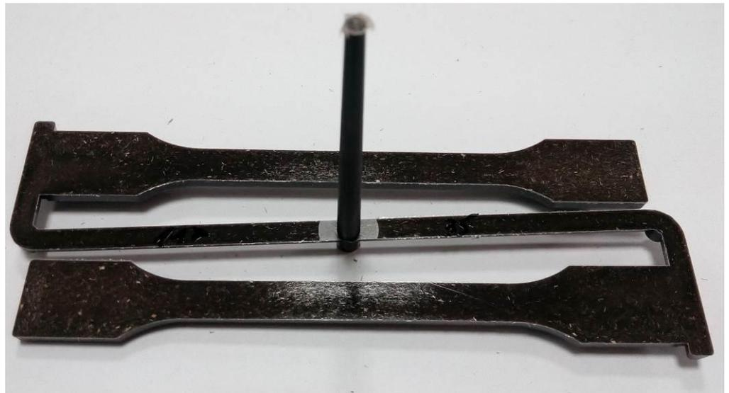
**Figure 2.** Samples made of PHBV–flax fiber biocomposite (30 wt.%).
