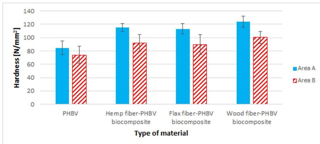
Figure 9. Hardness for pure polymers and biocomposites with various filler types for A and B areas.
