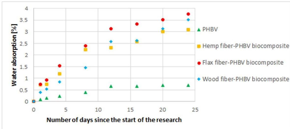
Figure 6. Water absorption for biocomposites with a variable type of filler and for pure PHBV.
