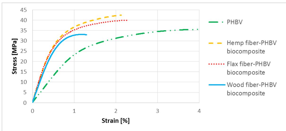
Figure 7. Stress–strain characteristics for pure PHBV and biocomposites with different types of filler.
