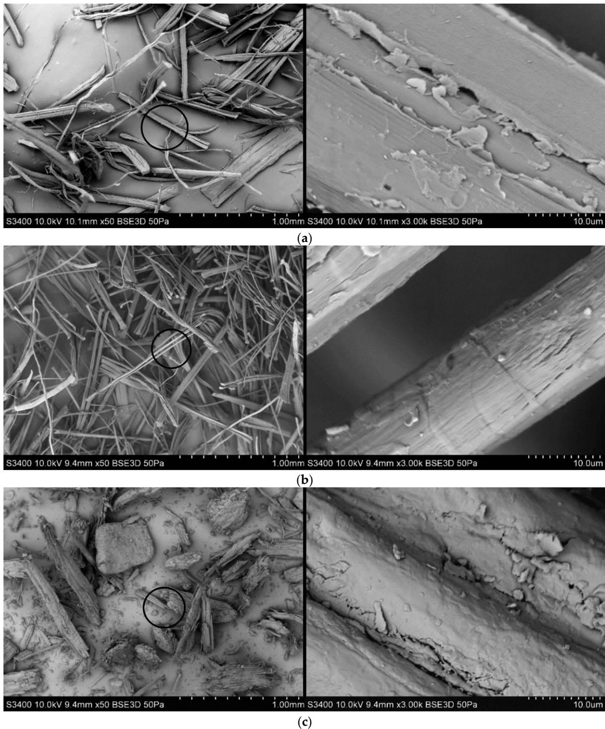
**Figure 1.** SEM photography of (a) hemp, (b) flax and (c) wood fibers.
