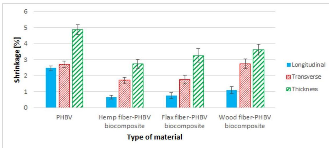
Figure 5. Shrinkage: longitudinal and transverse, in thickness for biocomposites with a variable type of filler and for pure PHBV biopolymer.
