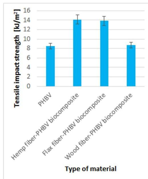
**Figure 8.** The results of tensile impact strength test for pure polymers and biocomposites with various fillers type.
