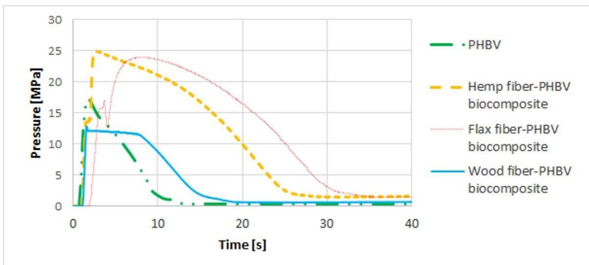
**Figure 3.** The pressure profile in mold cavity for biocomposites with a variable type of filler and pure biopolymer.
