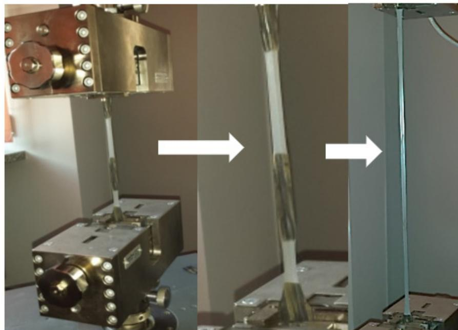
**Figure 7.** View of the sample during tensile test.
