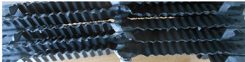
Figure 4. View of the filling packets of the cooling tower.
