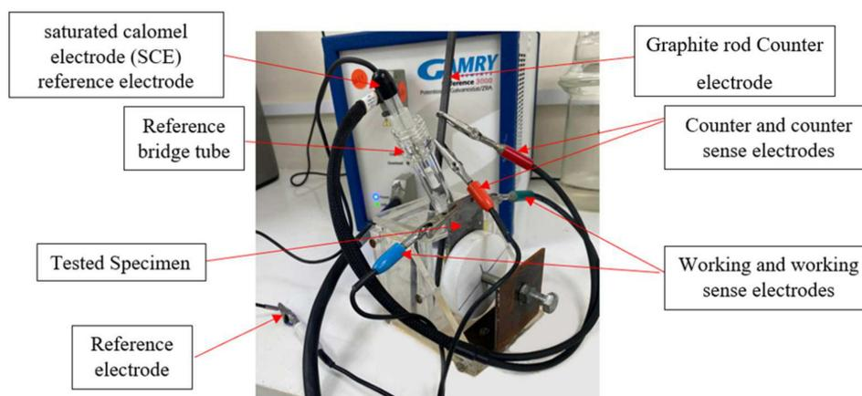
**Figure 3.** The electrochemical cell setup.
