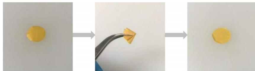
Figure 3. Twisting test of PI-CPE film.
