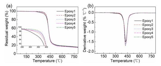
**Figure 6.** (a) Thermogravimetric Analysis (TGA) and (b) derivative thermogravimetric (DTG) curves of epoxy resins from room temperature to 800  $^{\circ}$ C under a nitrogen atmosphere with a heating rate of 10  $^{\circ}$ C/min.
