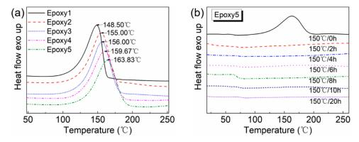
**Figure 3.** (a) Differential Scanning Calorimeter (DSC) curves of five uncured epoxy resin systems with different GA contents at the heating rate of 10  $^{\circ}$ C/min under a nitrogen atmosphere; (b) DSC curves of Epoxy5 after pre-cured at 100  $^{\circ}$ C for 2 h and post-cured at 150  $^{\circ}$ C for different hours at the heating rate of 10  $^{\circ}$ C /min under a nitrogen atmosphere.
