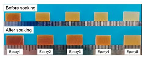
**Figure 8.** The appearance of epoxy resins with different crosslink densities before and after being soaked in TCB at 180  $^{\circ}$ C for 12 h.
