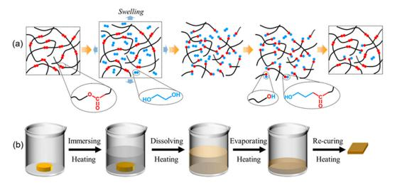
**Figure 1.** (a) The schematic of ethylene glycol (EG)-assisted dissolution and recycling mechanism: The crosslinked network is immersed in EG and heated, then alcohol molecules diffuse into the network and cleave ester bonds on the polymer skeleton. The repolymerization of decomposed epoxy oligomer occurs via evaporating excess EG. (b) The schematic illustration of the dissolution and recycling experiments.
