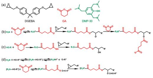
the participation of DMP-30, a crosslinked network structure containing a large number of ester bonds was formed by the curing reaction of anhydride and epoxy groups.
