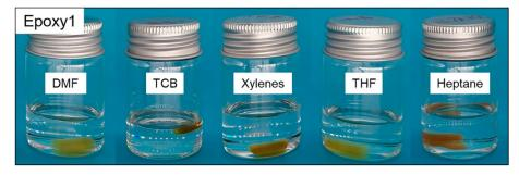
**Figure 7.** The appearance of Epoxy1 after being immersed in N,N-dimethylformamide (DMF), TCB, xylenes, tetrahydrofuran (THF), and heptane at ambient temperature for 96 h.
