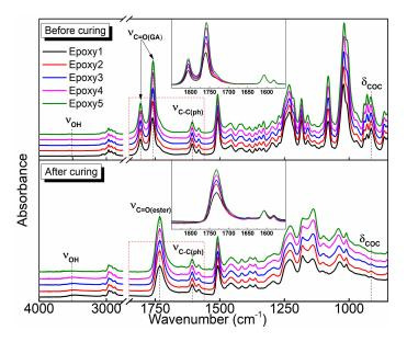
**Figure 4.** Fourier Transform Infrared Spectroscopy (FTIR) spectra of five epoxy systems with different contents of GA before and after curing. The curing condition is 100 °C for 2 h and then 150 °C for 6 h.
