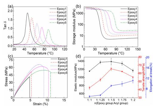
**Figure 5.** (a) Tan  $\delta$  curves as a function of temperature. Take the temperature corresponding to the peak of the curve to be  $T_g$ ; (b) Storage modulus curves of epoxy resins with different GA contents as a function of temperature; (c) Uniaxial tensile stress-strain curves of fresh epoxy resins; (d) The changes of elastic modulus, tensile strength, and elongation at break with the ratio of the epoxy group and acyl group.
