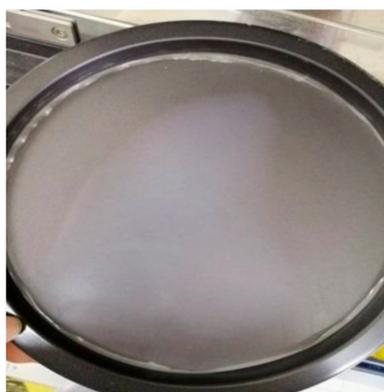
**Figure 1.** Dried film of the thermoplastic starch-dolomite (TPS-DOL) biocomposite in the Teflon-coated mould.
