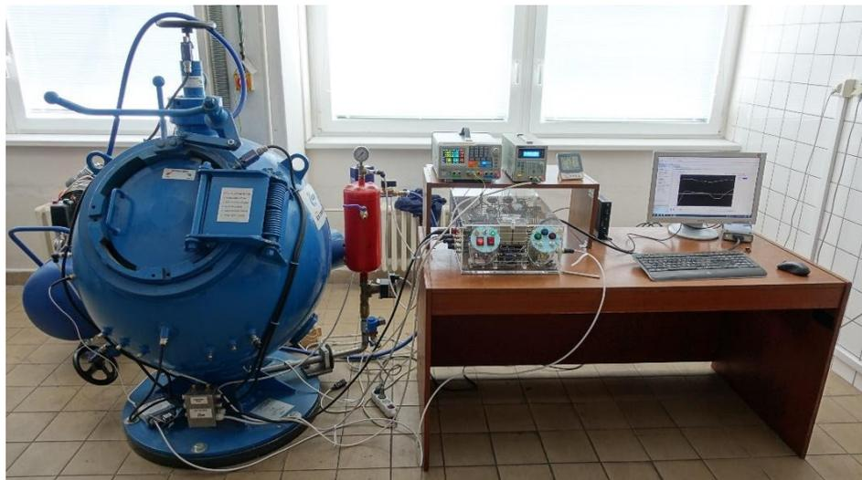
**Figure 7.** KV 150M2 explosion chamber.
