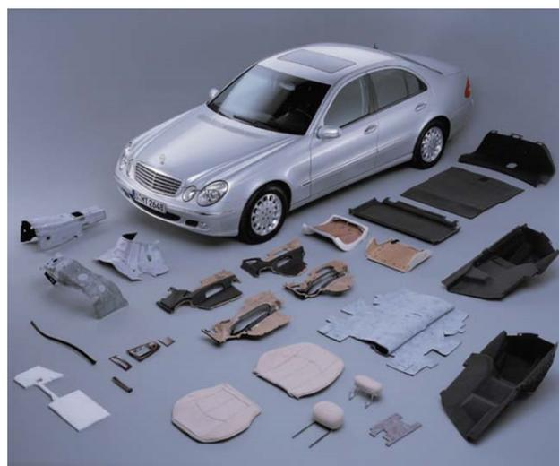
**Figure 1.** Examples of biocomposite applications in automobiles containing flax, hemp, sisal, and wool [26].
