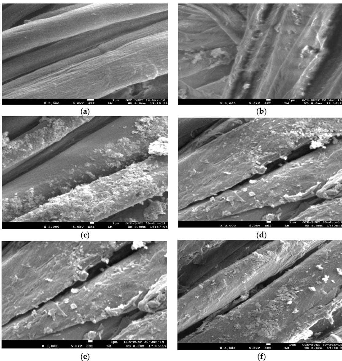
**Figure 8.** SEM images of different samples: (a) untreated fabric, (b) NanoZnO-1, (c) NanoZnO-2, (d) NanoZnO-3, (e) NanoZnO-2 after washing, and (f) NanoZnO-3 after washing.
