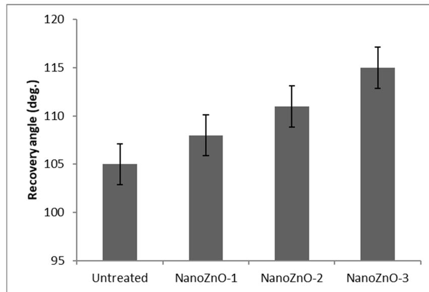
Figure 7. Crease recovery of untreated and ZnO nano-treated fabric.
