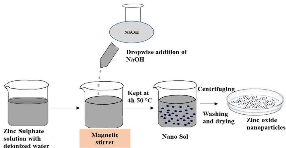
Figure 1. Experimental setup for the synthesis of ZnO nanoparticles.
