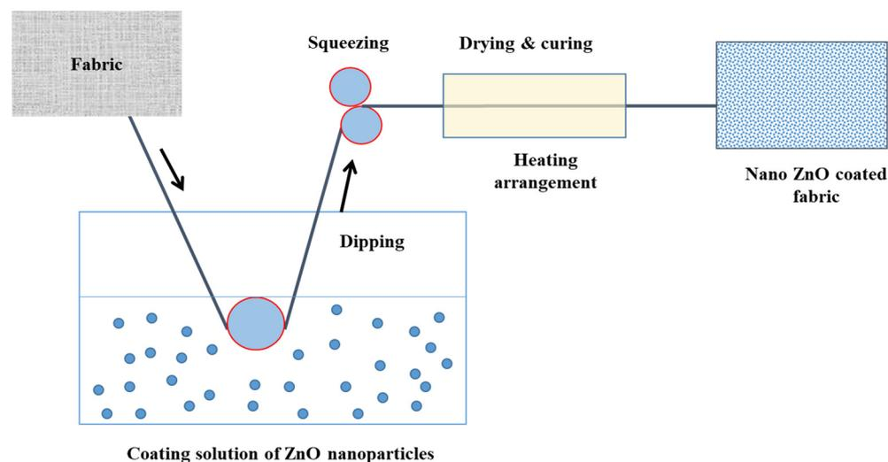
**Figure 3.** The sequence of thermo-fixation coating of nanoparticles on the fabric surface.
