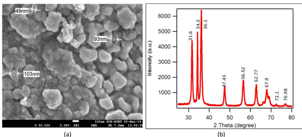
**Figure 2.** (a) SEM (scanning electron microscope) images of ZnO nanoparticles in  $\times 50,000$  magnification with size; (b) XRD (X-ray diffraction) pattern ZnO nanoparticles.
