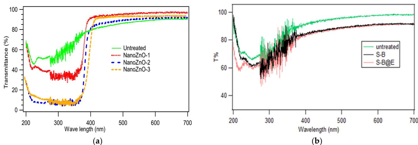
**Figure 4.** UV transmittance curve of (a) untreated fabric and different ZnO nano-coated fabric; (b) untreated fabric, only binder-treated (S-B) fabric, and binder with emulsifier-treated fabric (S-B@E).
