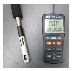
Figure 4. Hot wire anemometer.
