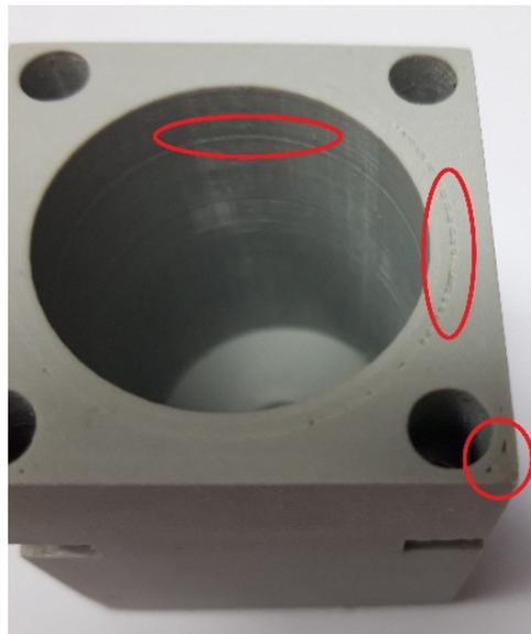
**Figure 2.** Errors on 3D printed test cylinder.
