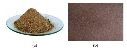
**Figure 3.** (a) Dry-compounded feedstock and (b) sample board, after hot-pressing at 180 °C for 30 min.
