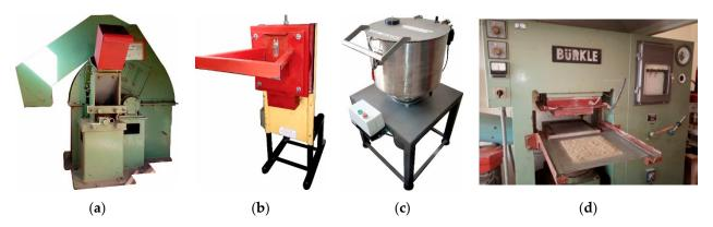
Figure 2. (a) Knife chipper, (b) hammermill, (c) custom-built blender, and (d) hydraulic press.
