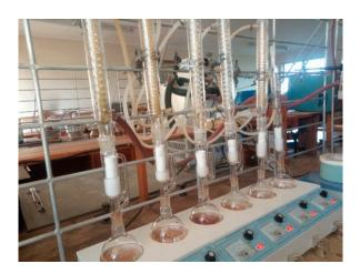
Figure 5. Soxhlet extraction setup for biomass compositional analysis.
