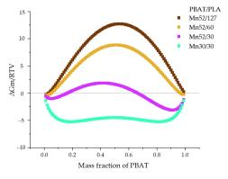
Figure 5. Phase diagram of PBAT/PLA blends with various molecular weights at 296 K.
