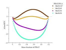
Figure 6. Phase diagram of PBAT/PLA blends with various molecular weights at 463 K.
