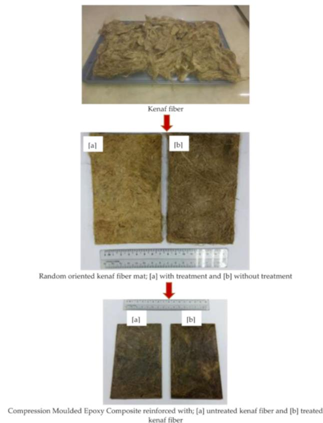
**Figure 3.** Compression moulded epoxy composites reinforced with untreated kenaf fiber and treated kenaf fiber.
