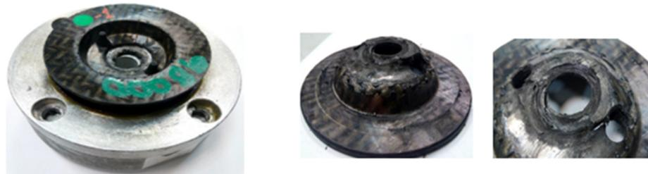
**Figure 12.** PA6-FG sheet: 3 mm CFRTP deformed after the fatigue test.
