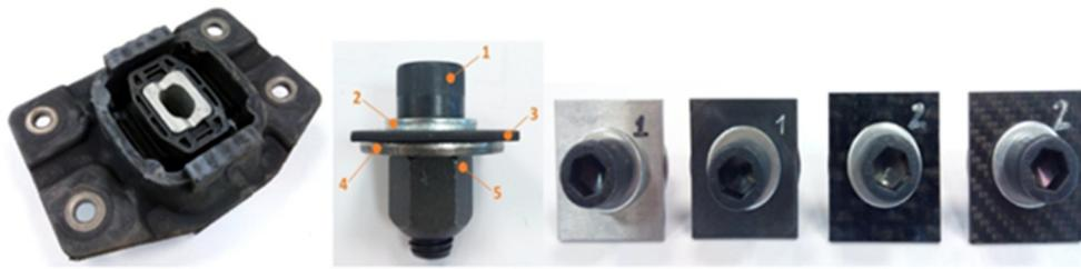
**Figure 2.** The torque test specimen assembly following a dry mounting configuration (bolt, nut, washers, metal part, and composite part).
