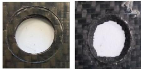
**Figure 6.** PA66-CF45 plate disassembled at a maximum: **(Left)** Produced by maximum tightening torque. **(Right)** Produced when applied torque is greater than maximum tightening torque.
