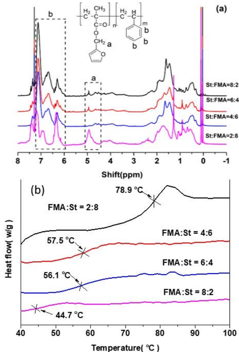
**Figure 3.** (a) <sup>1</sup>H NMR spectra and (b) DSC curves of copolymer P(St-co-FMA) with different monomer feeding ratio.
