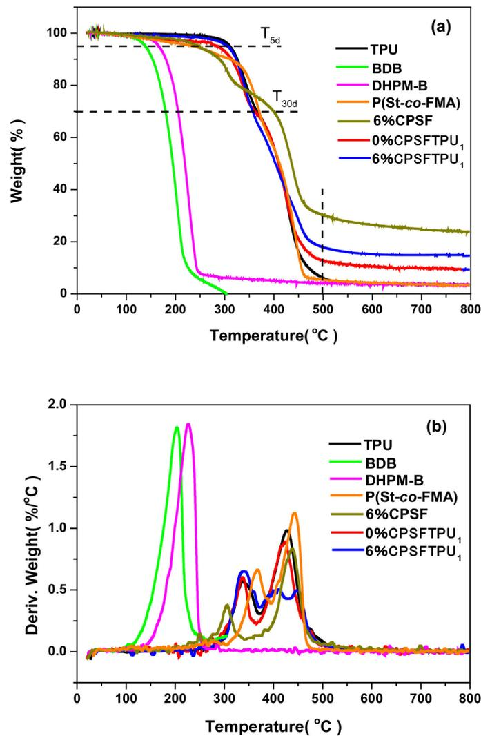
**Figure 10.** TGA (a) and DTG (b) curves of TPU, BDB, DHPM-B, P(St-co-FMA), 0%CPSTPU<sub>1</sub> and 6%CPSTPU<sub>1</sub>.
