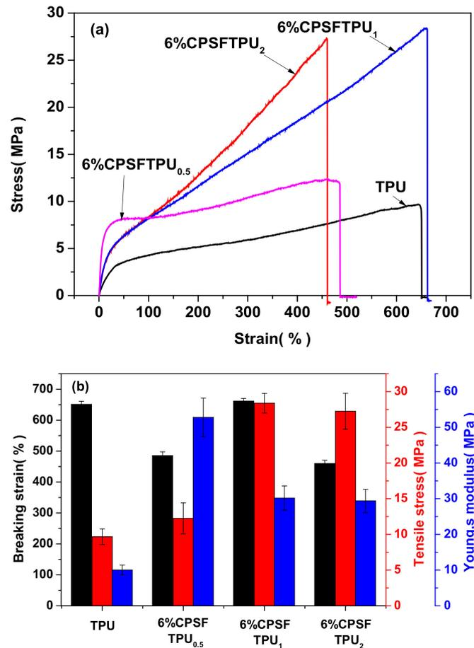
Figure 8. (a) Tensile curves and (b) mechanical properties of semi IPNs 6%CPSFTPU<sub>x</sub> series with different ratio of P(St-co-FMA)/TPU.
