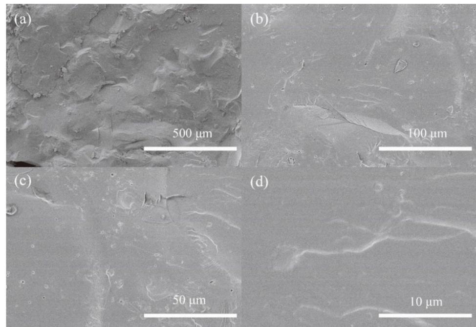
Figure 5. SEM images of semi IPNs 6%CPFSTPU<sub>1</sub> with different magnification times (a) 500 μm; (b) 100 μm; (c) 50 μm; (d) 10 μm.
