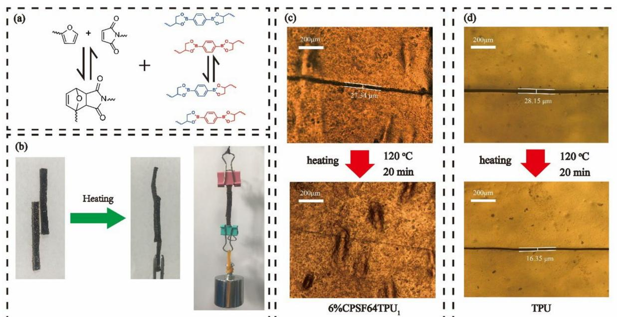
**Figure 11.** (a) Schematic representation of DA reaction (right) and the transesterification reaction of boronic ester linkages(right) (b) optical images of welding behaviors of 6%CPSFTPU<sub>1</sub> sample, optical microscope images of the and TPU fracture surface before and after self-healing: (c) for 6%CPSFTPU<sub>1</sub> and (d) for TPU.
