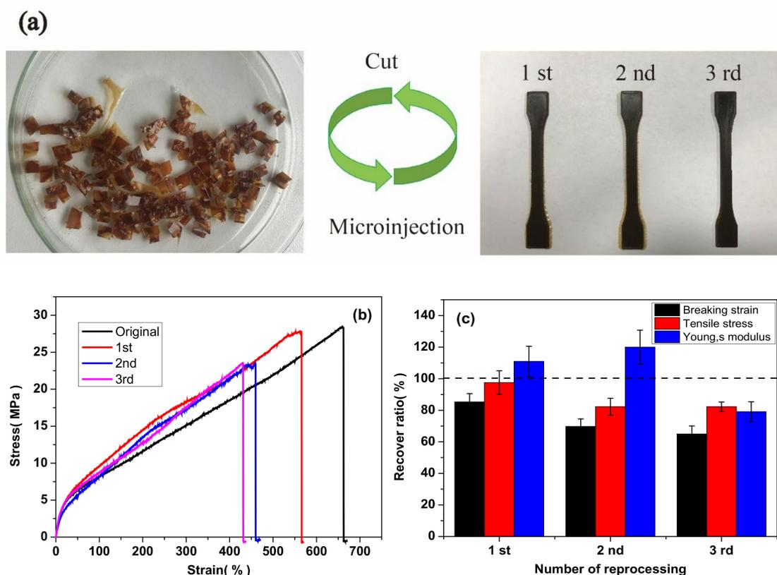
**Figure 13.** (a) Optical images of thermal recycling performance of semi IPNs 6%CPSTPU<sub>1</sub>, (b) mechanical properties of the samples with different generations: tensile curves and (c) recovery ratios.
