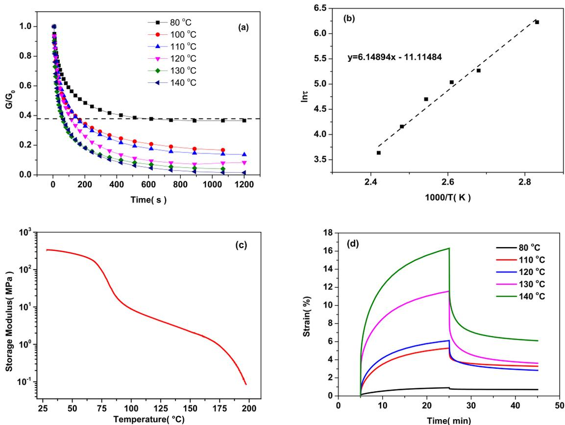
**Figure 7.** (a) Stress relaxation tests of the semi IPNs 6%CPSFTPU<sub>1</sub> at different temperatures, (b) Arrhenius plot with linear fit. From this fit the activation energy is calculated to be 55.3 kJ mol<sup>-1</sup>, (c) DMTA trace with a continually decreased storage modulus of semi IPNs 6%CPSFTPU<sub>1</sub>, (d) creep tests at different temperatures.
