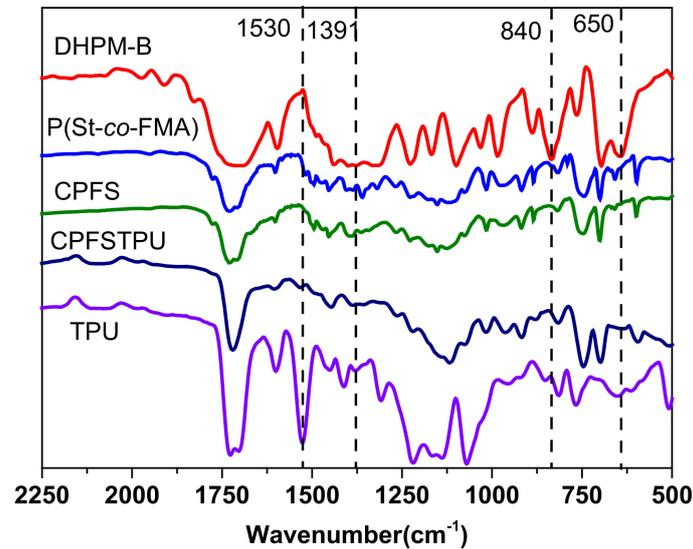
Figure 4. FTIR spectra of DHPM-B, P(St-co-FMA), CPFS, CPFSTPU and TPU.
