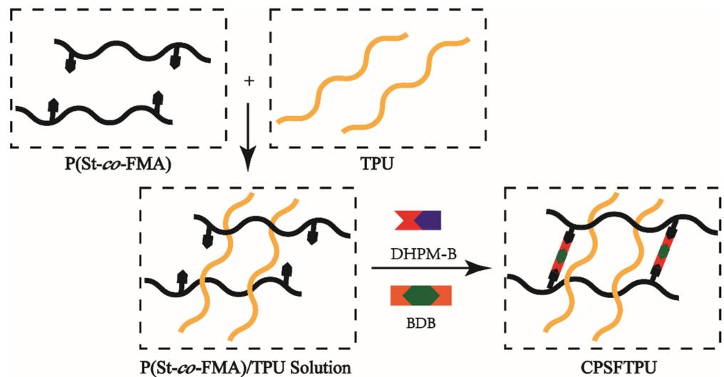
Figure 2. Preparation of semi IPNs of CPSFTPU.
