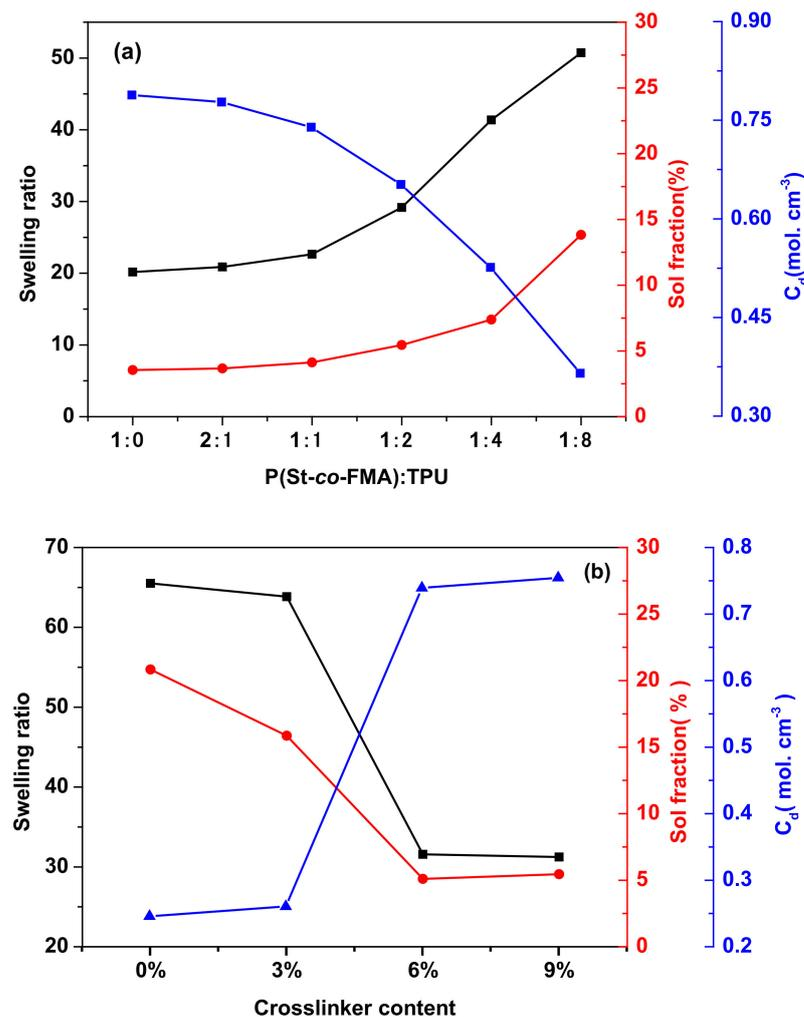
Figure 6. The swelling ratio, sol fraction and cross-link density of the semi IPNs series (a) with different ratios of P(St-co-FMA)/TPU, (b) with different crosslinker contents.
