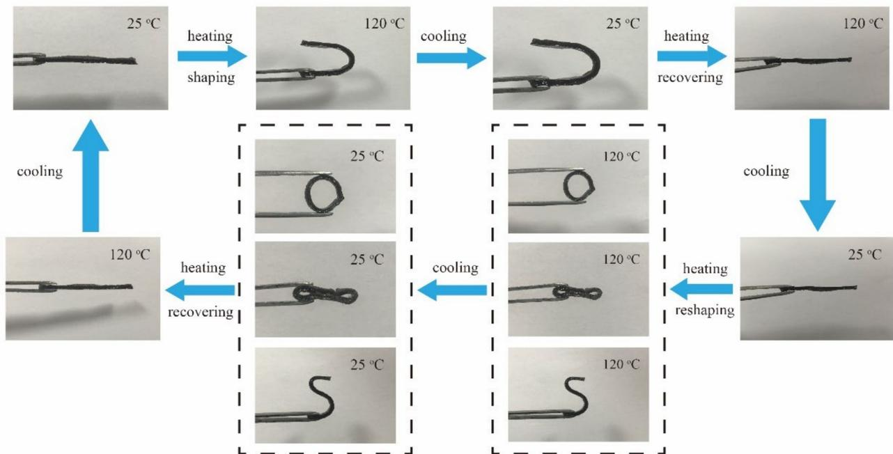
**Figure 12.** Optical images of shape-memory performance of the semi IPNs 6%CPSFTPU<sub>1</sub>.
