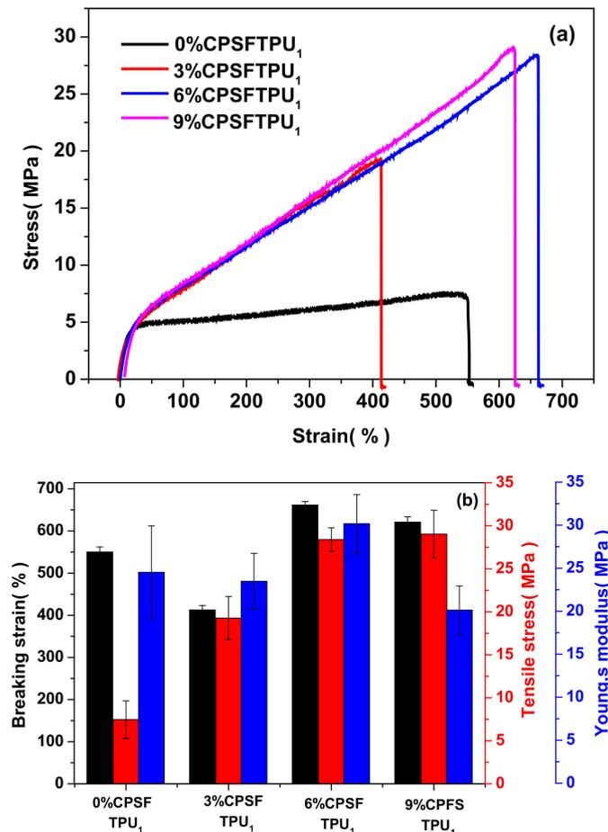
**Figure 9.** (a) Tensile curves and (b) mechanical properties of x%CPSFTPU<sub>1</sub> series with different crosslinker content.
