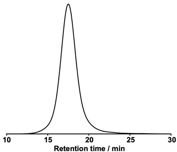
**Figure S2.** GPC chromatogram of PEG-PAsp (flow rate: 0.75 mL/min, eluent: 10 mM PB (pH 7.4), 150 mM NaCl, detector: UV at 220 nm).
