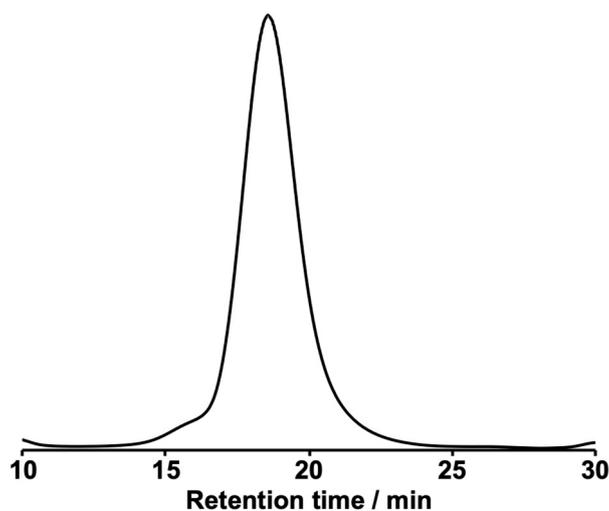
**Figure S4.** GPC chromatogram of PEG-P(Asp-AP) (flow rate: 0.75 mL/min, eluent: 10 mM Acetic acid, 500 mM NaCl, detector: UV at 220 nm)
