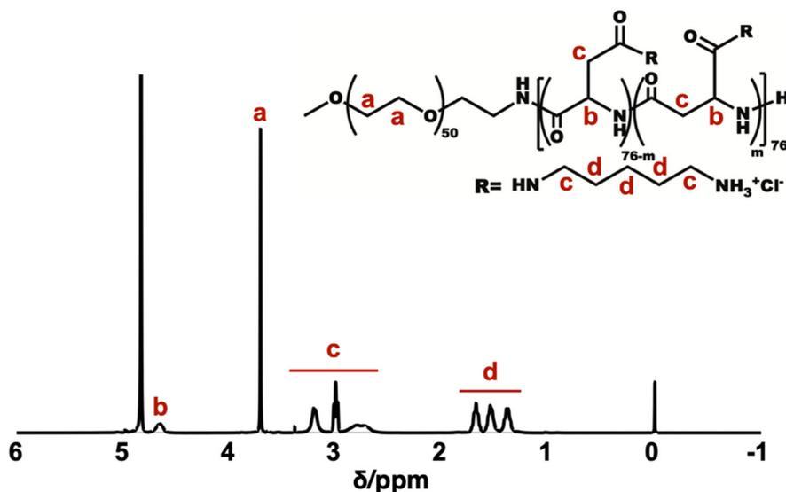
**Figure S3.** <sup>1</sup>H-NMR spectrum of PEG-P(Asp-AP) (solvent: D<sub>2</sub>O, temperature: 25 °C)
