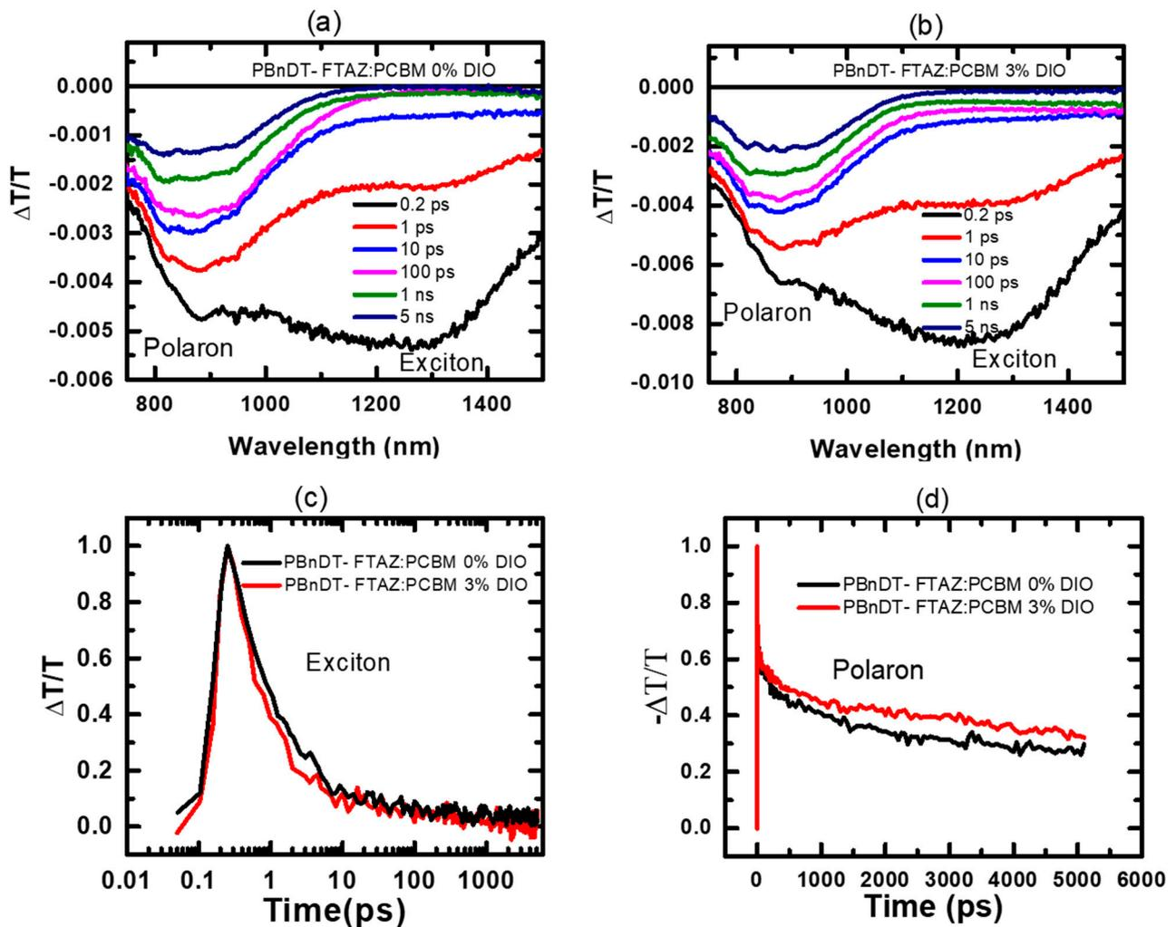
**Figure 3.** Transient absorption spectra of PBnDT-FTAZ:PCBM blend films with (a) 0% DIO and (b) 3% DIO, and comparison of (c) exciton and (d) charge separation dynamics.
