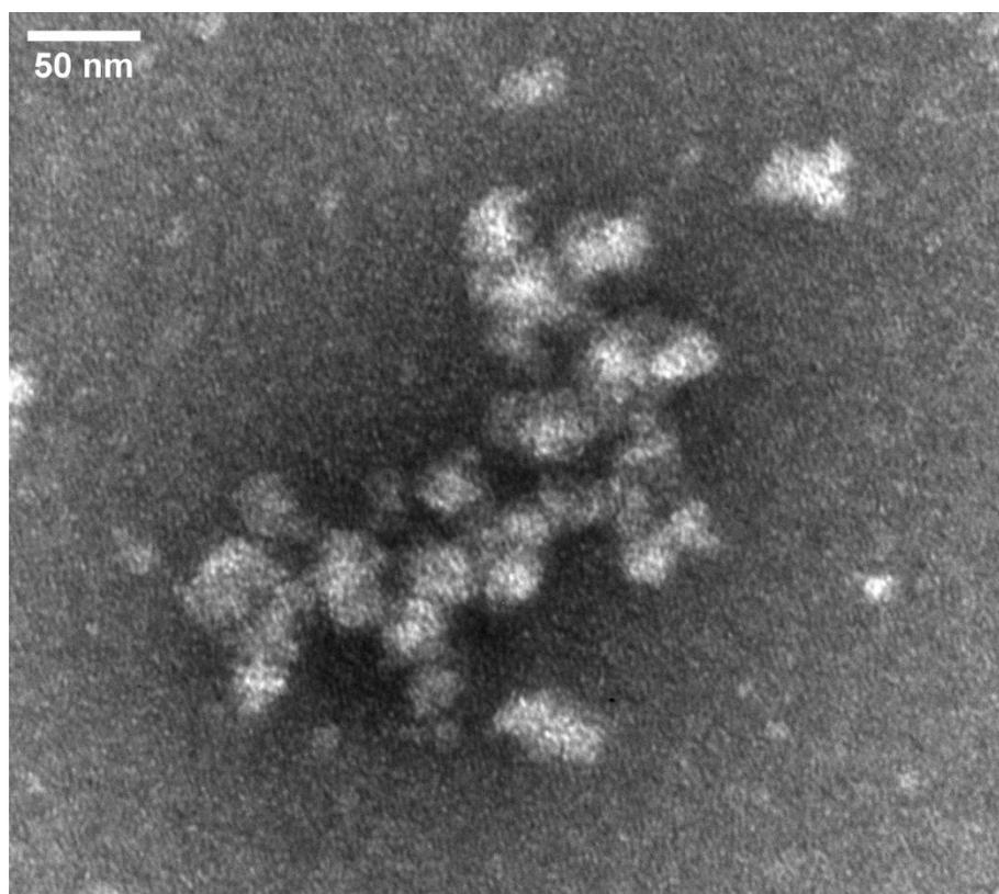
**Figure S12:** TEM micrograph of nanogels N50 taken at 80 KeV.
