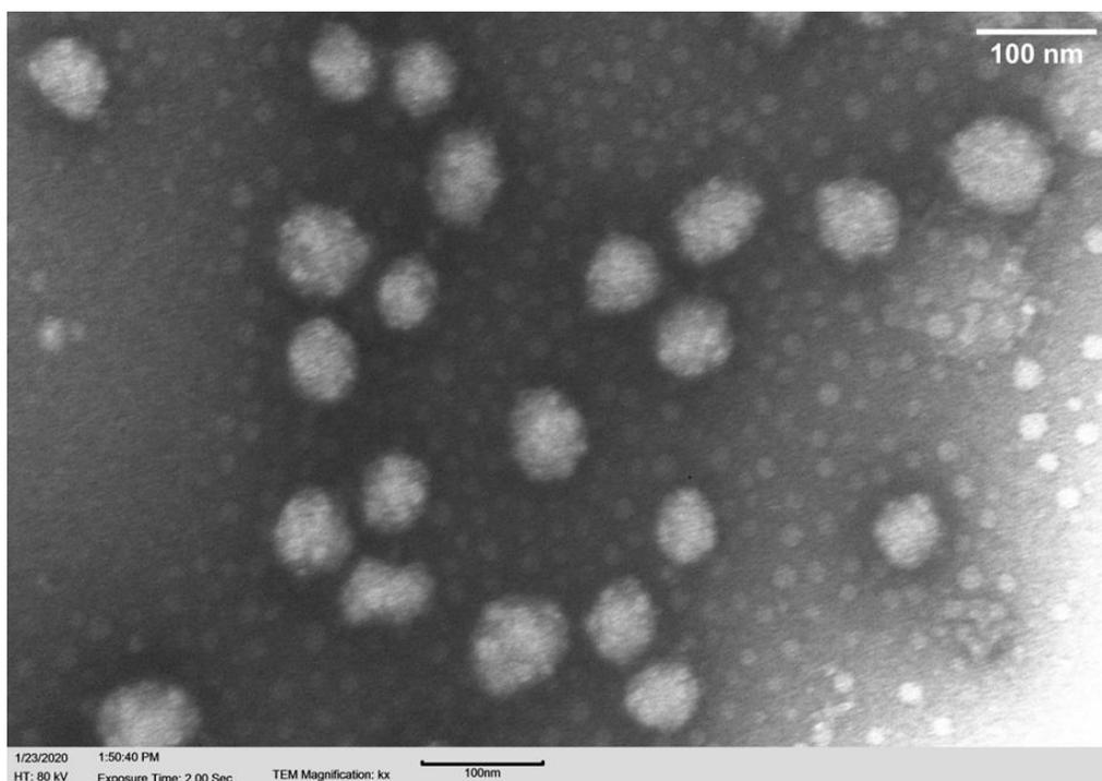
**Figure S13:** TEM-micrograph of nanogels N48 taken at 80 KeV.
