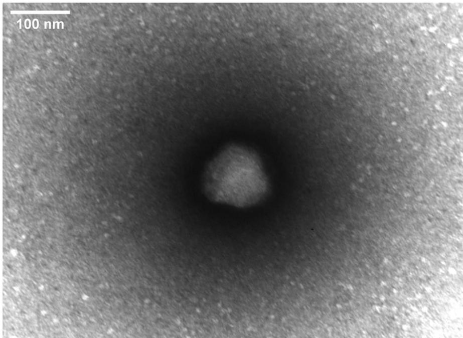
**Figure S10** TEM micrograph of nanogel N42 taken at 80 KeV.
