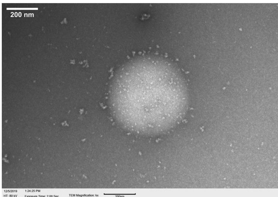
**Figure S11:** TEM-micrograph of nanogels N32 taken at 80 KeV.
