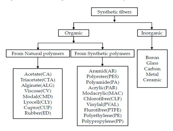
Figure 5. Classification of synthetic fibers [15].
