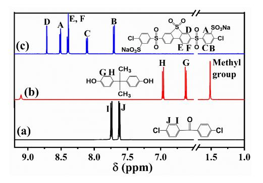
Figure S1. <sup>1</sup>H NMR spectra of (a) DCBP, (b) BPA and (c) sBCPSBP. The monomers were dissolved in DMSO-d<sub>6</sub> for <sup>1</sup>H NMR analysis.
