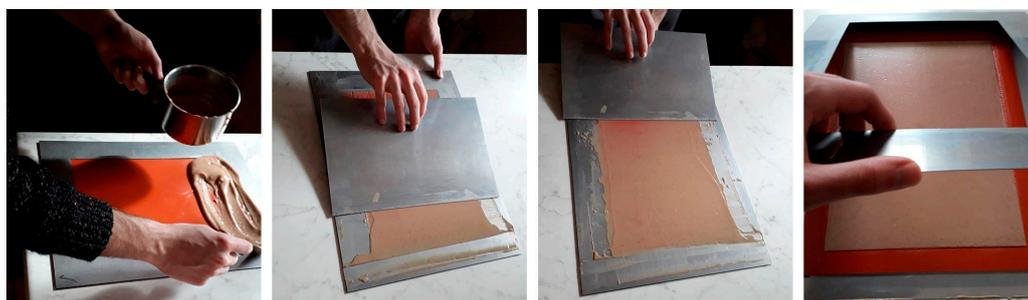
Figure 2. The different phases of the film casting.
