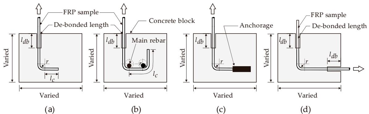
**Figure 3.** Different pullout setups for examining the bend capacity of FRP reinforcements; (a) J-hook specimen, (b) U-shaped specimen, (c) J-hook specimen with anchorage, and (d) J-hook specimen with unbonded unloaded end (illustration adopted from [38]).
