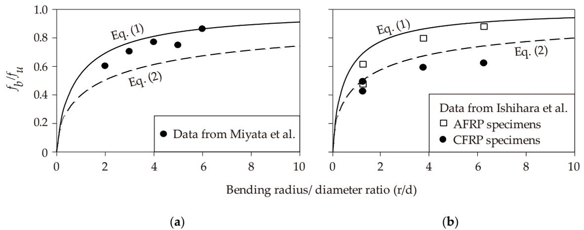
**Figure 7.** Predicted bend capacity of FRP bars from Nakamura and Higai’s (a) and Ishihara et al.’s (b) models.
