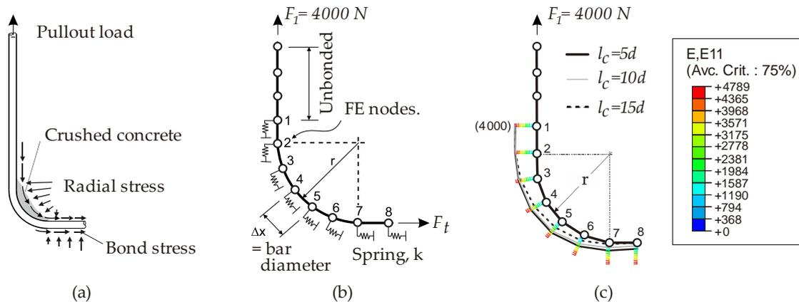
**Figure 4.** Physical model vs. mathematical finite element (FE) model for a bent FRP bar; (a) pullout test on J-hook FRP bar, (b) modelling of bond along FRP/concrete interface, and (c) strain distribution along the bent portion of FRP bar.
