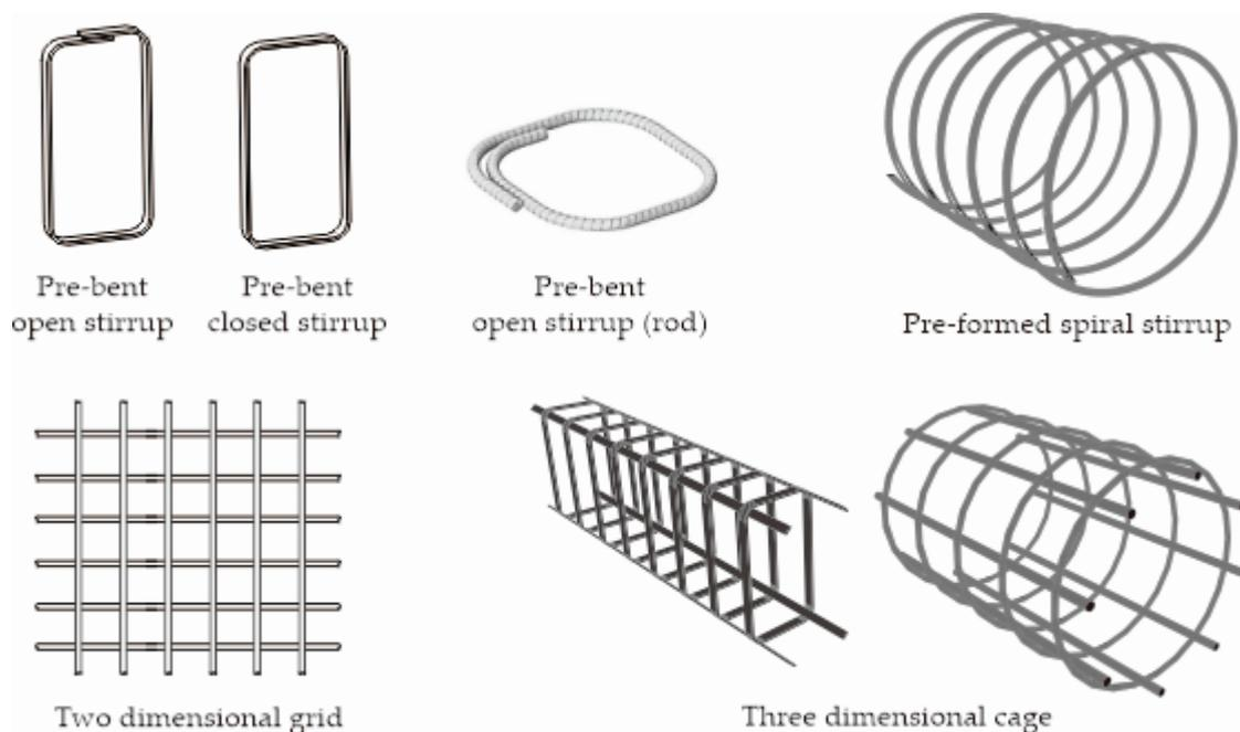
**Figure 10.** Various commercially available shaped FRP reinforcements (adopted from [38]).
