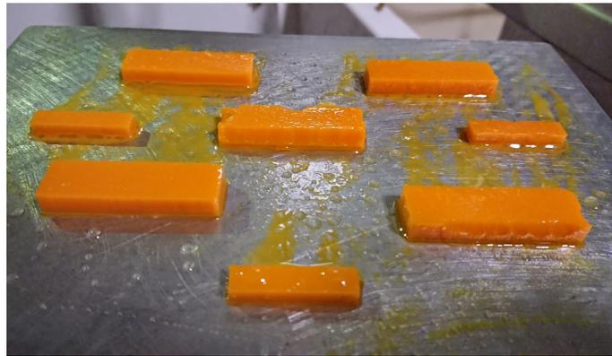
**Figure 5.** Printing trials for the CE7030 blend with the optimized printing conditions after photocuring optimization (see Table 2).
