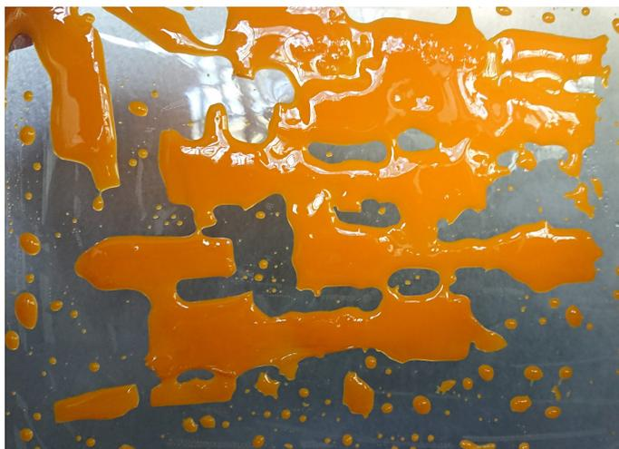
**Figure 4.** Printing trials for the CE7030 blend with the same printing conditions used for the cream resin (see Table 2).
