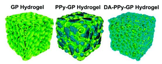
**Figure 2.** A schematic of structure and morphology for an elastomeric gelatin methacrylate-polyacrylamide (GP) double network hydrogel, polypyrrole (PPy) incorporated GP hydrogel, and dopamine (DA)-PPy-GP hydrogel. Reproduced with permission from [59]. Copyright 2019, Royal Society of Chemistry.
