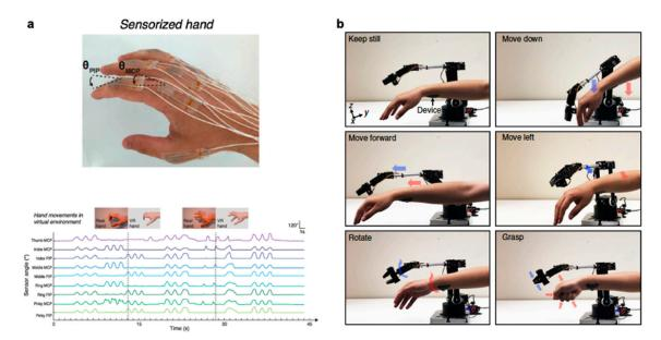
**Figure 21.** (a) Hand movement tracking for virtual reality applications [252]. Adapted and reproduced with permission as licensed under the Creative Commons Attribution 4.0 International License. (b) Wireless robotic arm control with electromyograph (EMG) data acquired from various arm motions. Reproduced with permission from [24]. Copyright 2017, Springer Nature.
