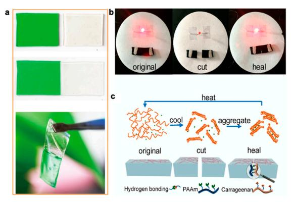
**Figure 7.** (a) Demonstration of a glycerol/hydroxyethycellulose (GHEC) macromolecular elastomeric gel self-healing through presence of dynamic hydrogen bonds [197]. Adapted and reproduced with permission as licensed under the Creative Commons Attribution 4.0 International License. (b) Self-healing ability of the dual conductive network hydrogel. (c) Schematic of the self-healing mechanism. Adapted with permission from [198]. Copyright 2020, American Chemical Society.
