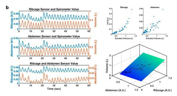
**Figure 20.** (a) Demonstration of sensor placement for ribcage and abdomen along with attachment setup. (b) Representative signals from ribcage and abdomen plotted with simultaneous respiration volume along with scatterplots for each [6]. Adapted and reproduced with permission as licensed under the Creative Commons Attribution 4.0 International License.
