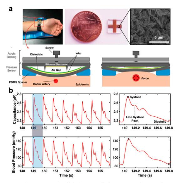
**Figure 18.** (a) Demonstration of wrinkled gold capacitive blood pressure sensor placement and set-up along with (b) corresponding arterial pulse waveforms for beat-to-beat measurements. Reproduced with permission from [8]. Copyright 2019 John Wiley and Sons.
