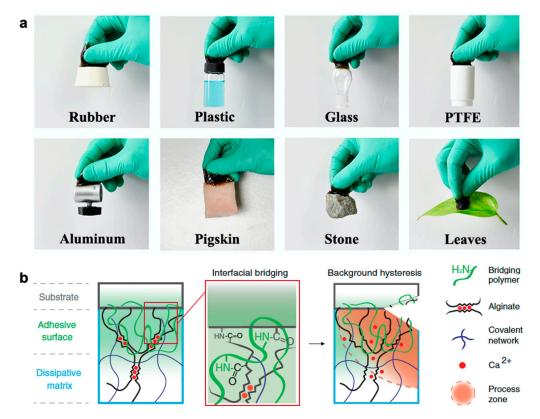
**Figure 8.** (a) Demonstration of PDA-based hydrogel adhesion to various materials. Adapted with permission from [210]. Copyright 2019, American Chemical Society. (b) Design schematic for a hydrogel-based tough adhesive inspired by slug mucus which shows how the bridging polymer can be absorbed to the tissue surface through electrostatic attractions and allow for covalent bonding [214]. Copyright 2017, The American Association for the Advancement of Science.
