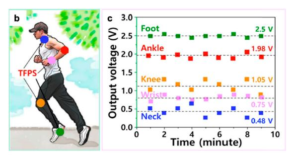
**Figure 14.** (a) Output voltage demonstration of TFPS with movement of foot, neck (voice vibration), wrist, and knee. (b,c) Schematic of device placement on a running individual along with stability tests at the corresponding locations. The statistical results were recorded nine times for 10 min under identical conditions. Reproduced with permission from [235]. Copyright Elsevier 2018.
