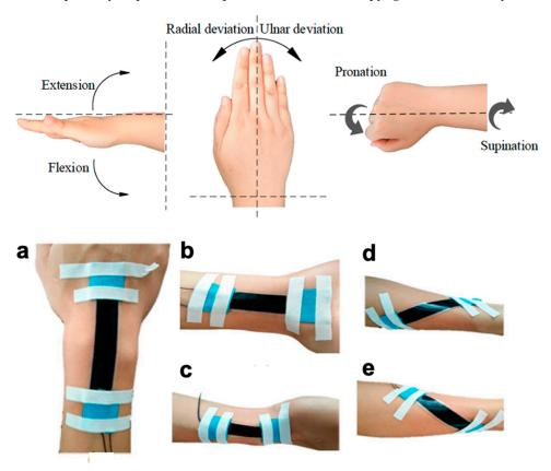
**Figure 10.** Decomposition of possible wrist motions for the wrist joint along with corresponding placement of a capacitive motion sensor for tracking of (a) flexion (b) extension (c) Ulnar deviation (d) pronation (e) supination [222]. Reproduced with permission as licensed under the Creative Commons Attribution 4.0 International License.
