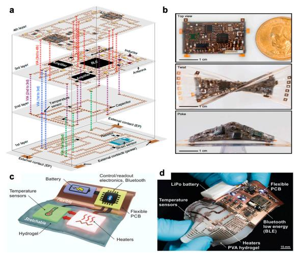
**Figure 23.** (a) Exploded schematic of a four-layer electronic system and (b) demonstration of the system's ability to withstand mechanical deformation. Reproduced with permission from [24]. Copyright 2019, Springer Nature. (c) Concept and (d) photograph of hydrogel electronic skin [64]. Adapted and reproduced with permission as licensed under the Creative Commons Attribution 4.0 International License.
