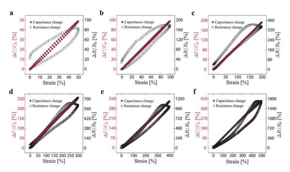
**Figure 6.** Comparison of capacitive and resistive strain sensor response for carbon black-filled elastomers under different strain amplitudes for (a) 50% (b) 100% (c) 200% (d) 300% (e) 400% and (f) 500% strain. Visible hysteresis can be seen in the resistive response between loading and unloading strain. Reproduced with permission from [167]. Copyright 2017, John Wiley and Sons.
