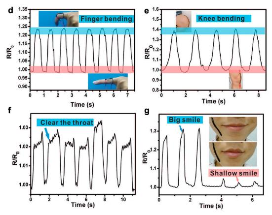
**Figure 11.** (a–c) Demonstration of PVA/PDA hydrogel compliance, fluidity, and self-adhesion to fingertip. Motion detection demonstration of the PVA/PDA hydrogel with (d) finger bending, (e) knee bending, (f) throat movement, and (g) smiling. Reprinted with permission from [230]. Copyright 2018 The Royal Society of Chemistry.
