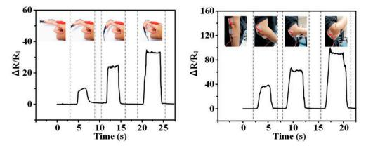
**Figure 9.** Demonstration of a resistive strain sensor using overlapped CNTs to track bending of the finger and elbow, respectively. Reproduced with permission from [221]. Copyright 2019, John Wiley and Sons.
