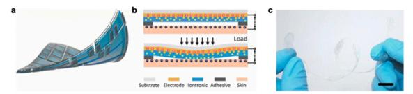
**Figure 19.** (a) Perspective view and (b) cross-sectional view of the epidermal-iontronic interface device. Reproduced with permission from [122]. Copyright 2018, John Wiley and Sons. (c) Photo of an iontronic pressure sensor array. Scale bar is 1 cm. Reproduced with permission from [125]. Copyright 2015, Springer Nature.
