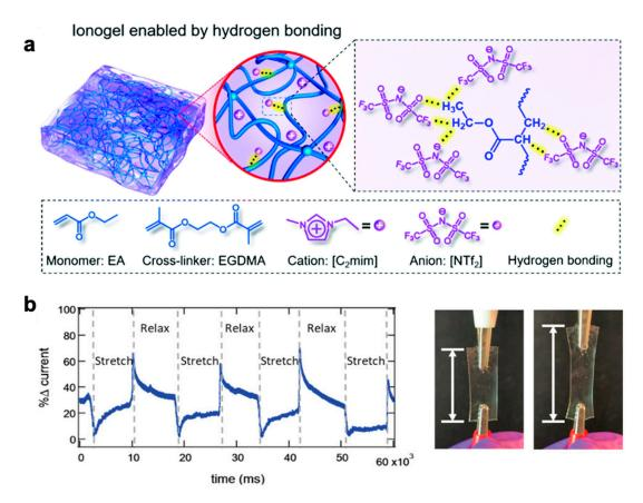
**Figure 5.** (a) Schematic description of a transparent, mechanically robust, and stable ionogel enabled by hydrogen bonding. Reproduced with permission from [128]. Copyright 2020, Royal Society of Chemistry (b) Mechanical characterization of a 3D printed crosslinked ionogel. Reproduced with permission from [129]. Copyright 2019, John Wiley and Sons.
