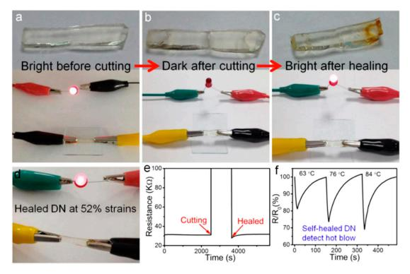
**Figure 16.** (a–c) Demonstration of the self-healing conductivity for a double network hydrogel before and after cutting and after self-healing. (d) The double network hydrogel remains conductive at 52% strain after self-healing. (e) Resistive time-evolution of the self-healing process. (f) Demonstration of dynamic response to different temperatures after self-healing. Reprinted with permission from [22]. Copyright 2018 American Chemical Society.
