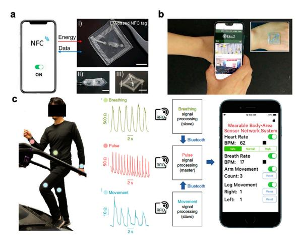
**Figure 24.** (a) Liquid metal-based hydrogel NFC tag with demonstrated use (b). Reproduced with permission from [111]. Copyright 2020 John Wiley and Sons. (c) Demonstration of bodyNET system with corresponding signal outputs for breathing, pulse, and arm movement. Reprinted with permission from [238]. Copyright 2019, Springer Nature.
