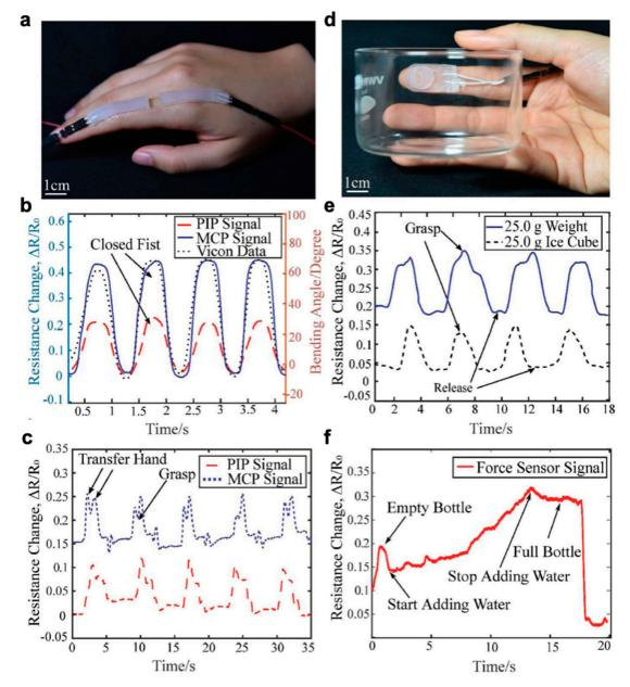
**Figure 13.** Demonstration of various functionalities as wearable sensors for hand motion detection with strain sensing along the proximal interphalangeal (PIP) joint and metacarpophalangeal (MCP) joint (a–c) and force sensing at the index fingertip for picking up items of different temperature (d,e) and force sensing of dynamic motions (f). Reproduced with permission from [234]. Copyright 2018 John Wiley and Sons.
